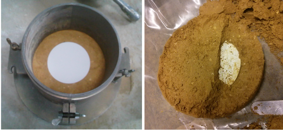
Figure B.1: Suction measurement on earthen cylindrical samples.
