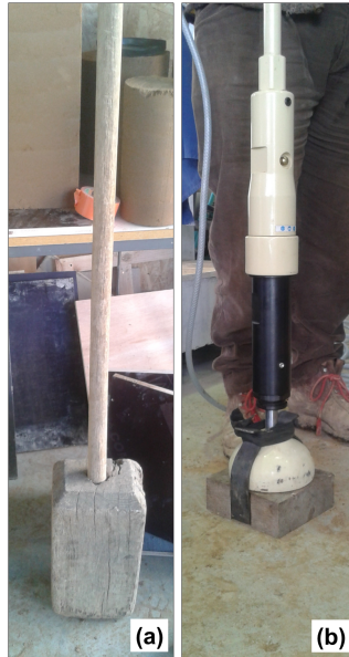
Figure 1.10: (a) Manual rammer in wood; (b) Pneumatic rammer with a wooden sabot.
