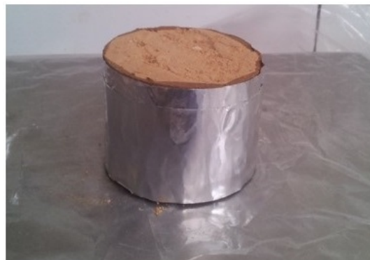
Figure 5.14: Sealing the lateral faces with paraffin and foil.
