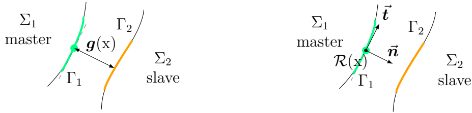
(a) Definition of the gap \mathbf{g} , orthogonal to the grey dashed line that is tangent to \Gamma_1 . (b) Example of a local referential \mathcal{R}(x) that is defined regarding to \Gamma_1 .
