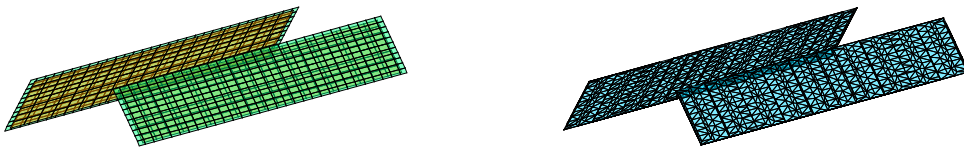
(a) Superposition of the blade and hub interfaces \Gamma_1 and \Gamma_2 (b) Transfer interface \Gamma built from the blade and hub interfaces
