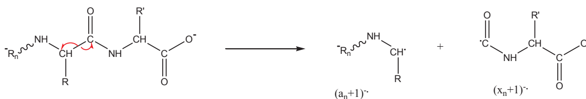
Scheme 2.2 Proposed mechanism for the formation of (a_n+1)^{\cdot-} and (x_n+1)^{\cdot-} fragment ions during UVPD of doubly deprotonated peptide [M-2H]^{2-} .
