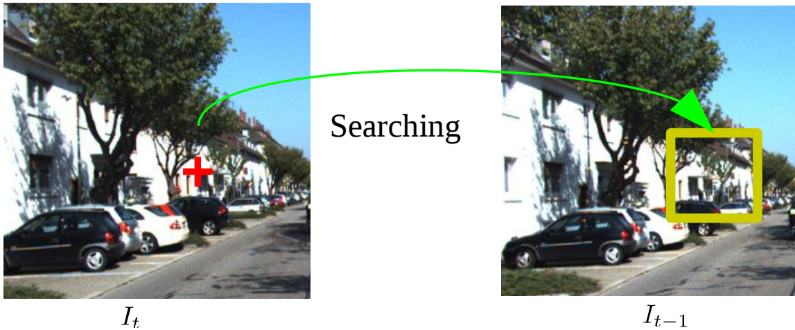
Figure 4.11: Matching for monocular case. Red cross in I_t represents the new interest point, the yellow rectangle is the searching area we expect to find the correspondence of the new interest point.
