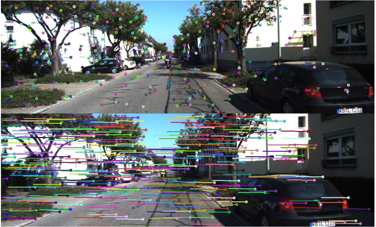
Figure 4.15: Matching of a stereo pair. The top image is the captured by left camera and the bottom one is the right image. The start points and searching scope in epipolar line for the interest points in left image are drawn with same color.
