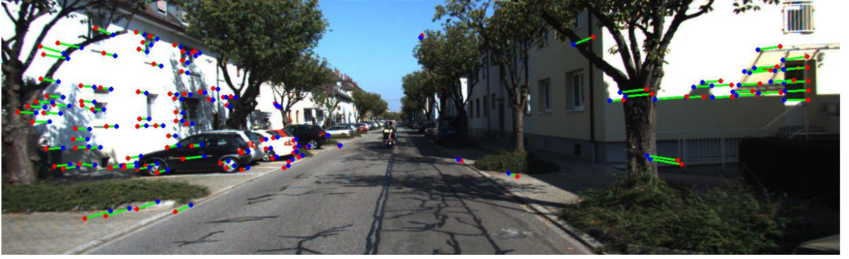
Figure 4.12: Existing correspond points between I_t and I_{t-1} . Red circle: the locations of image points in I_{t-1} . Blue circle: Matches of achieved by guided matching in section 4.3. Green lines: displacements of pixels.
