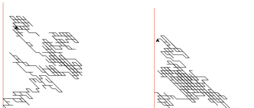
Figure 11.3: Two uniformly sampled Gouyou-Beauchamps walks on 800 steps: an unweighted (balanced) model (left) and a weighted (reluctant) model with parameters a = \frac{1}{\sqrt{2}} and b = 1 (right), which can be scaled into a model with weights of 1 and 2 by multiplying each weight by \sqrt{2} .
