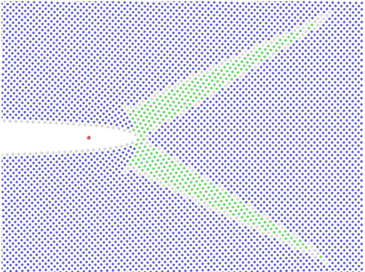
Figure V.51: The structural evolution of an initially equilibrium (010)[001] crack in bcc iron under additional deformation equal to +0.33\varepsilon_{yy(\infty)}^{Upper} , and after relaxation of 4 \times 10^4 time steps. The initial half-length of the crack was equal to 50 lattice parameters and the initial position of the crack-tip is denoted by a red circle. The crack propagates via brittle cleavage on the (010) crack plane and along the [100] direction. The blue and green colour atoms represent the bcc and fcc crystal structure, respectively.
