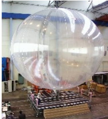
Figure 2.1 – Picture of a fully pressurized SPB similar to those used in this work.
