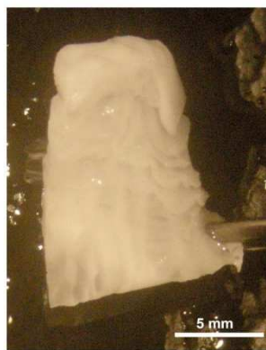
Figure 1. Light micrograph of 700 \mu\text{m} thick PCL (poly( \epsilon -caprolactone)) electrospun-nanofiber scaffold.
