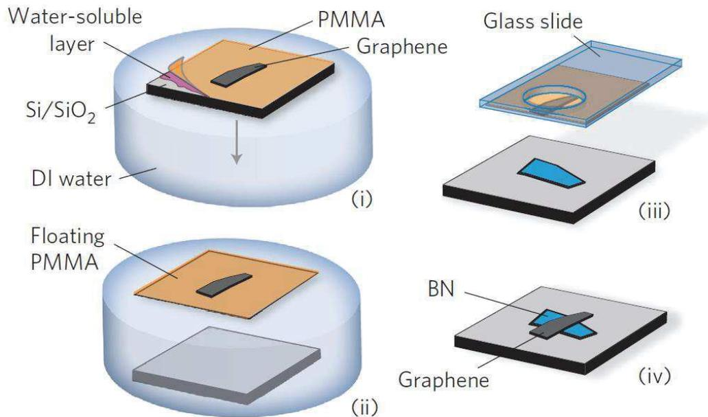
FIGURE 7.1: Four steps process that has been used to fabricate graphene-hBN hetero-structures. Figure taken from [219].
