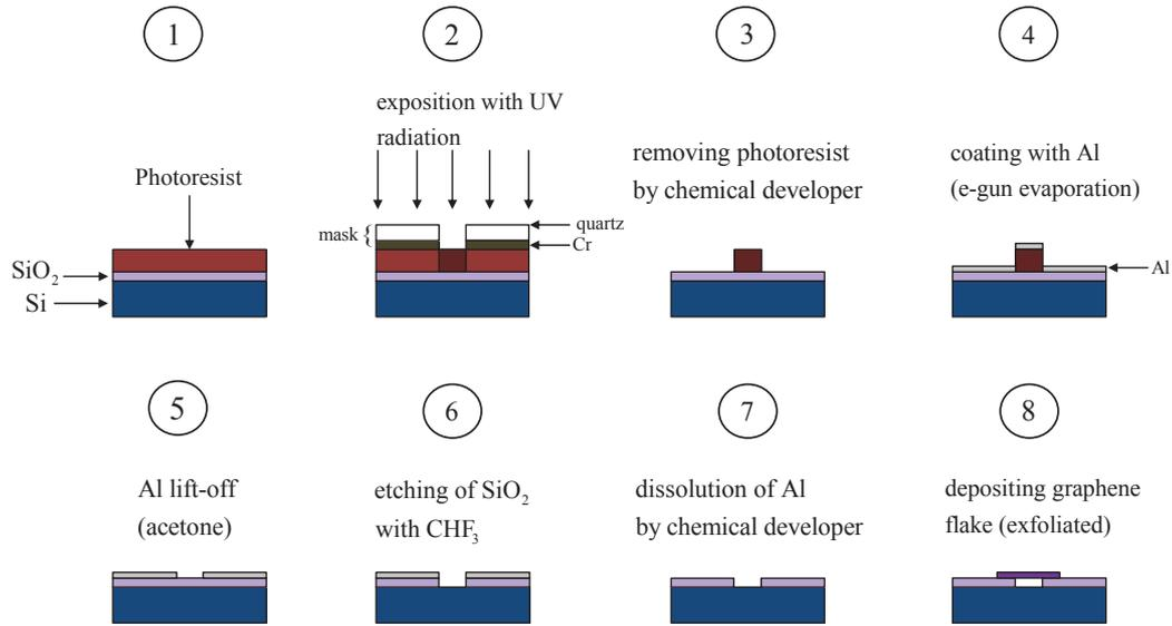
FIGURE 7.6: Schematic presentation of the 8 steps process to obtain suspended flakes of graphene over the silicon substrate.
