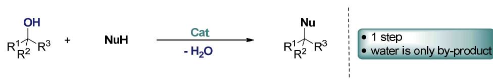
Scheme 1.3. Direct dehydrative substitution of alcohols.
