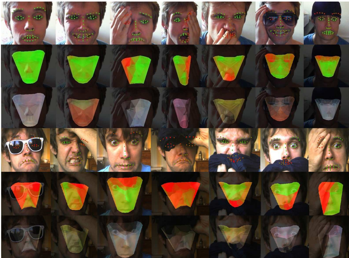
Figure 5.11: Examples of local FER under realistic occlusions. Top rows: point-wise confidence scores (red: low confidence, green: high confidence). Middle rows: triangle-wise scores. Bottom rows: weighted local classification (transparent for low confidences, gray for neutral, red for happy , yellow for angry , blue for sad , cyan for fear , green for disgust and magenta for surprise ). Best viewed in color.
