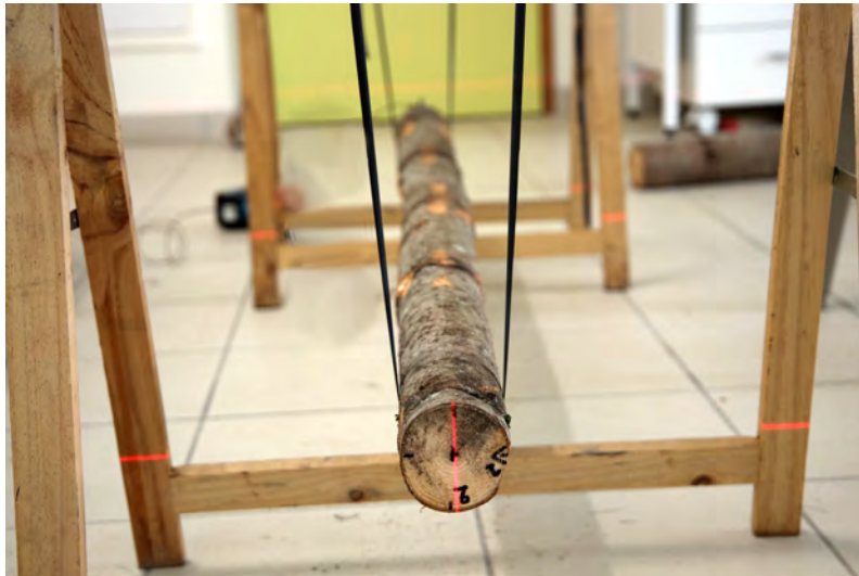
FIGURE 2.3 – Test bench for the MOE measurement
