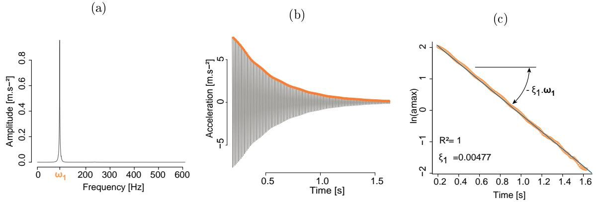
FIGURE 2.5 – Successive steps of the signal numerical treatment for  $\xi$  calculation. Example is given for mode 1. (a) FFT of the raw signal filtered by a pass-band filter centred on  $\omega_1$  (92.2 Hz). (b) first mode filtered acceleration (grey curve) and the maxima  $a_{max}(t)$  (orange dots). (c) Natural logarithm of the maxima  $\ln(a_{max}(t))$  with its linear regression. The slope of this regression divided by the pulsation  $\omega_1$  allows to calculate  $\xi_1$ .
