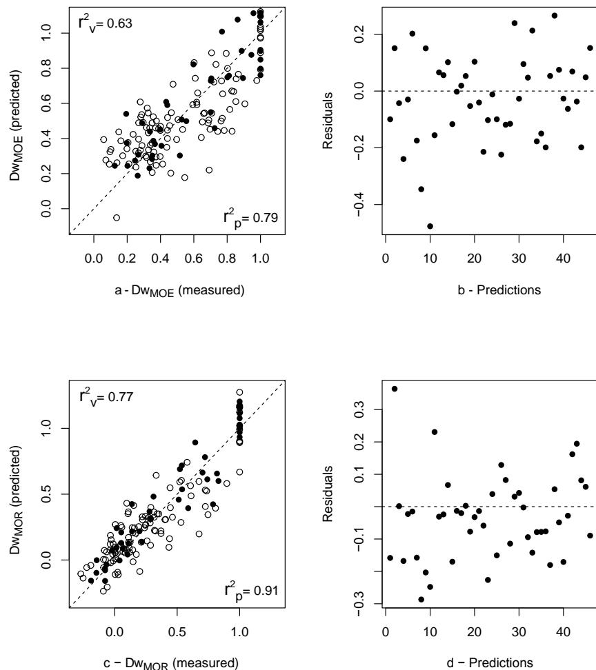
FIGURE 2.12 – Comparison between measured and predicted values for  $Dw_{MOE}$  (a) and  $Dw_{MOR}$  (c). The empty dots indicate the calibration set and the filled dots indicate the validation set. Prediction residuals  $Dw_{MOE}$  (b) and  $Dw_{MOR}$  (d) of for the validation set.
