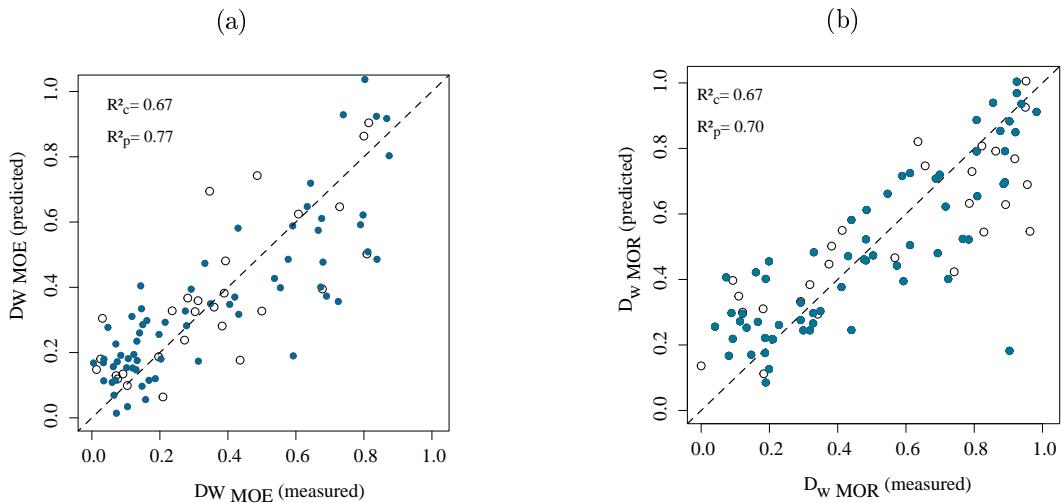
FIGURE 3.7 – (a) Measured  $Dw_{MOE}$  compared to predicted  $Dw_{MOE}$ . (b) Measured  $Dw_{MOR}$  compared to predicted  $Dw_{MOR}$ . The filled dots correspond to the calibration phase and the empty dots to the validation phase
