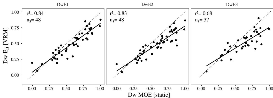
FIGURE 3.7 – Comparison of indicators of the level of decay  $Dw_{MOE}$  and  $Dw_{E_n}$  assessed by static method ( $Dw_{MOE}$ ) and VRM ( $Dw_{E_n}$ ). The black lines correspond to regression lines. The dashed lines correspond to the line of equality and  $n_s$  to the number of samples.
