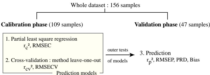
FIGURE 2.2 – Details on the validation process of the predictive models.
