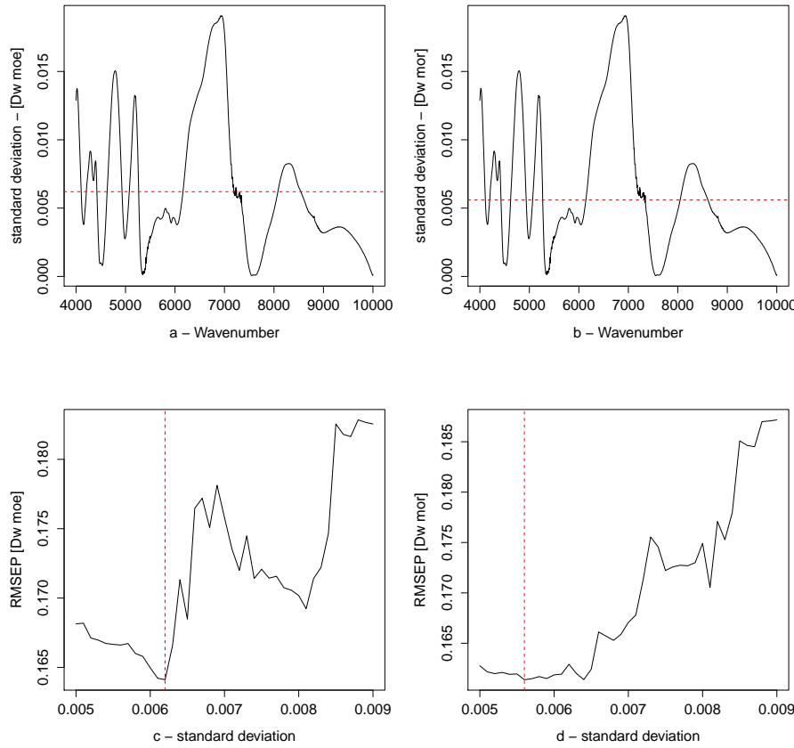
FIGURE 2.10 – Standard deviation of the differential spectra  $S_{diff}$  with the optimal  $SD_{lim}$  (red dashed lines) for PLSR with  $Dw_{MOE}$  (a), and with  $Dw_{MOR}$  (b). RMSEP variation is a function of  $SD_{lim}$  for  $Dw_{MOE}$  (c) and for  $Dw_{MOR}$  (d). The red dashed lines correspond to the optimal  $SD_{lim}$ , i.e. where RMSEP is minimal.
