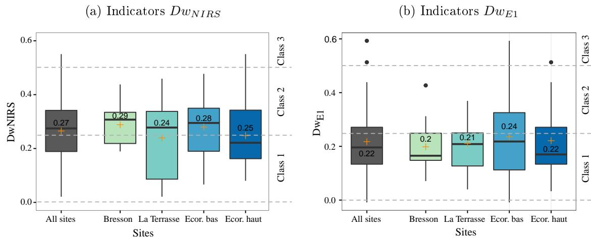
FIGURE 2.9 – Indicators of level of decay measured on 60 logs decayed in natural conditions. Results are shown all sites together (grey boxplot) and according the experimental sites. Crosses associated to figures correspond to the mean values of each indicators.
