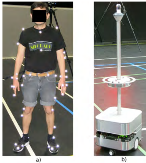
Figure 1.2: a) One of the participants equipped with the full body marker set. b) the mobile robot Robulab10.
