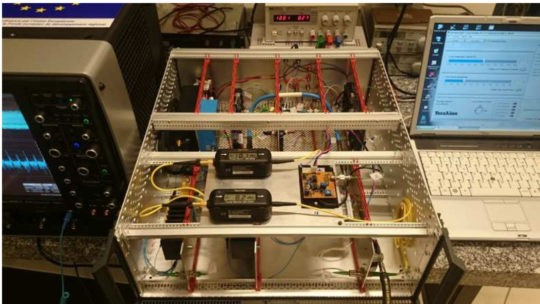
Figure 3.1: Picture of the photonic RC setup based on an EO phase delay dynamics.
