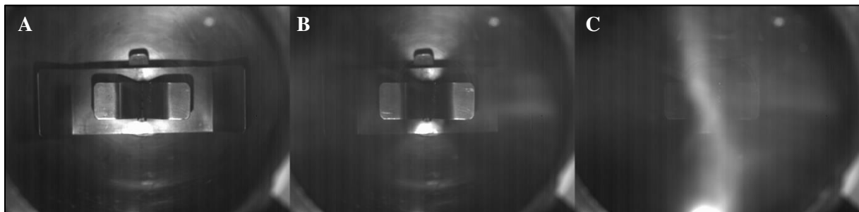
Figure 3.36. Injection of a combustible dust developed with the standard rebound nozzle
