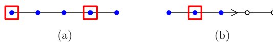
Figure 3.3: (a) A dominating set of P_5 with two vertices. (b) One vertex is enough to power dominate P_5 : ultimately, propagation allows to monitor all vertices.
