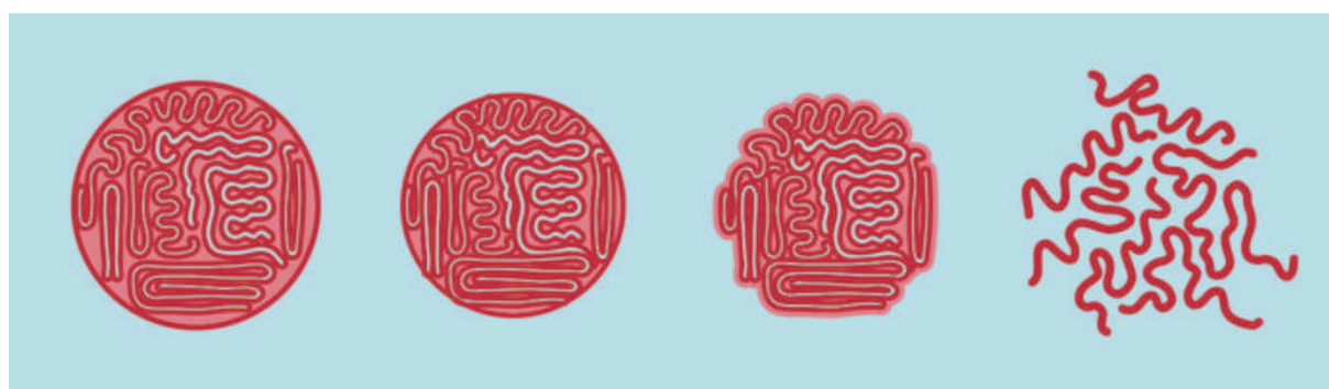
Figure 17 Schematic representation of the formation of elongated PS-PEO micelles. The solvent is evaporating from left to right. The dark red represents the PS blocks. Evaporation of the chloroform will cause the confinement of the elongated water domains. This continues until a sponge phase is formed. Finally reducing the solvent even more will cause an emulsion inversion which results in the formation of PS-PEO cylinders in water.
