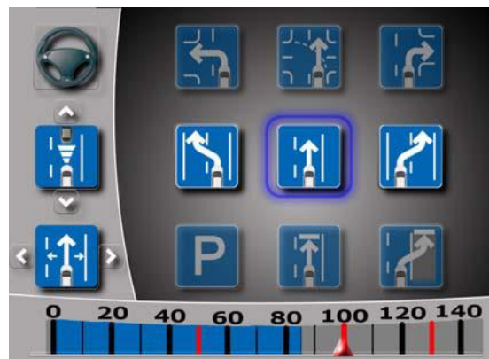
Figure 2.2 Tactile touch display of a maneuver interface in the “Conduct-by-wire” project (Franz et al. 2012)
