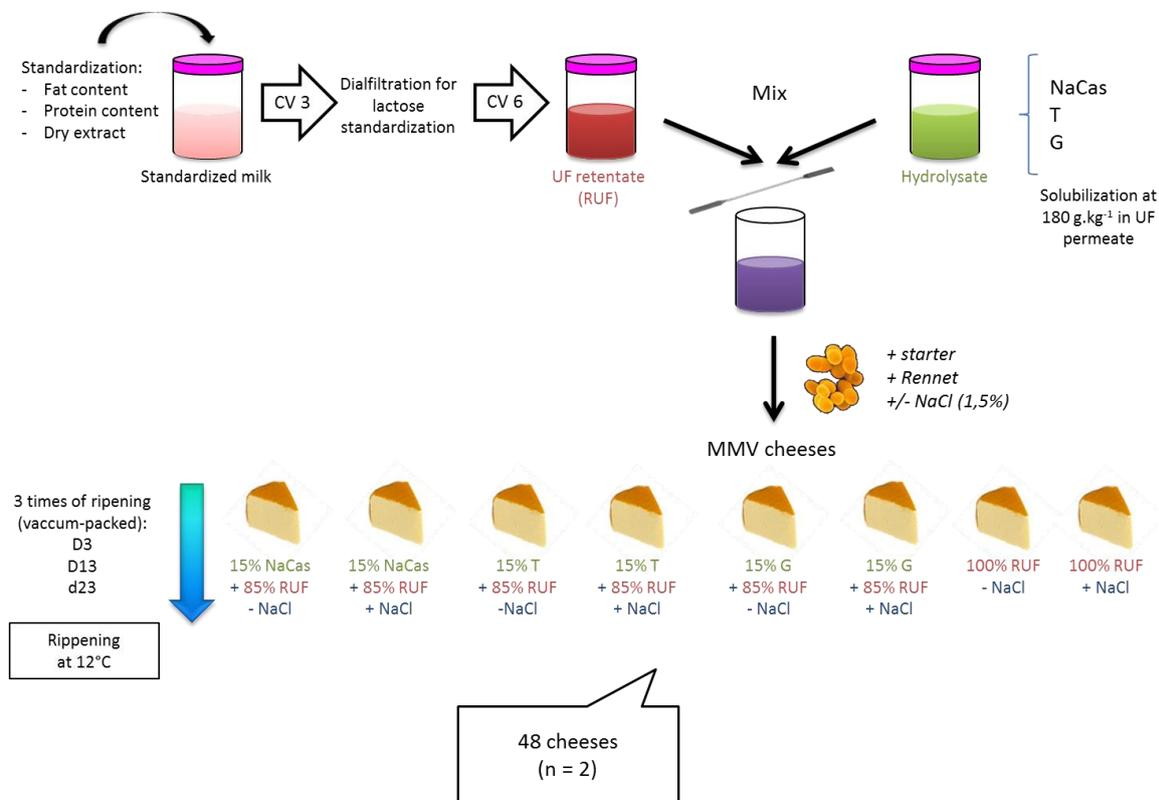
Fig 1. Manufacture of MMV cheeses with addition of hydrolysates (Tryptic or Glu-C hydrolysates) or sodium caseinate (NaCas).
