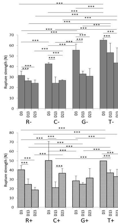
Fig. 8. Rupture strength of cheeses at 3 (D3), 13 (D13) and 23 (D23) days of ripening. Cheeses are manufactured with ultrafiltrate retentate (R) used as a control, and with 15% (w/w) sodium caseinate (C), Trypsin hydrolysate (T) and Glu-C hydrolysate (G), with (+ in light grey) or without (- in dark grey) NaCl. The mean and SEM are represented; \*  $P < 0.05$ ; \*\*  $P < 0.01$ ; \*\*\*  $P < 0.001$ .
