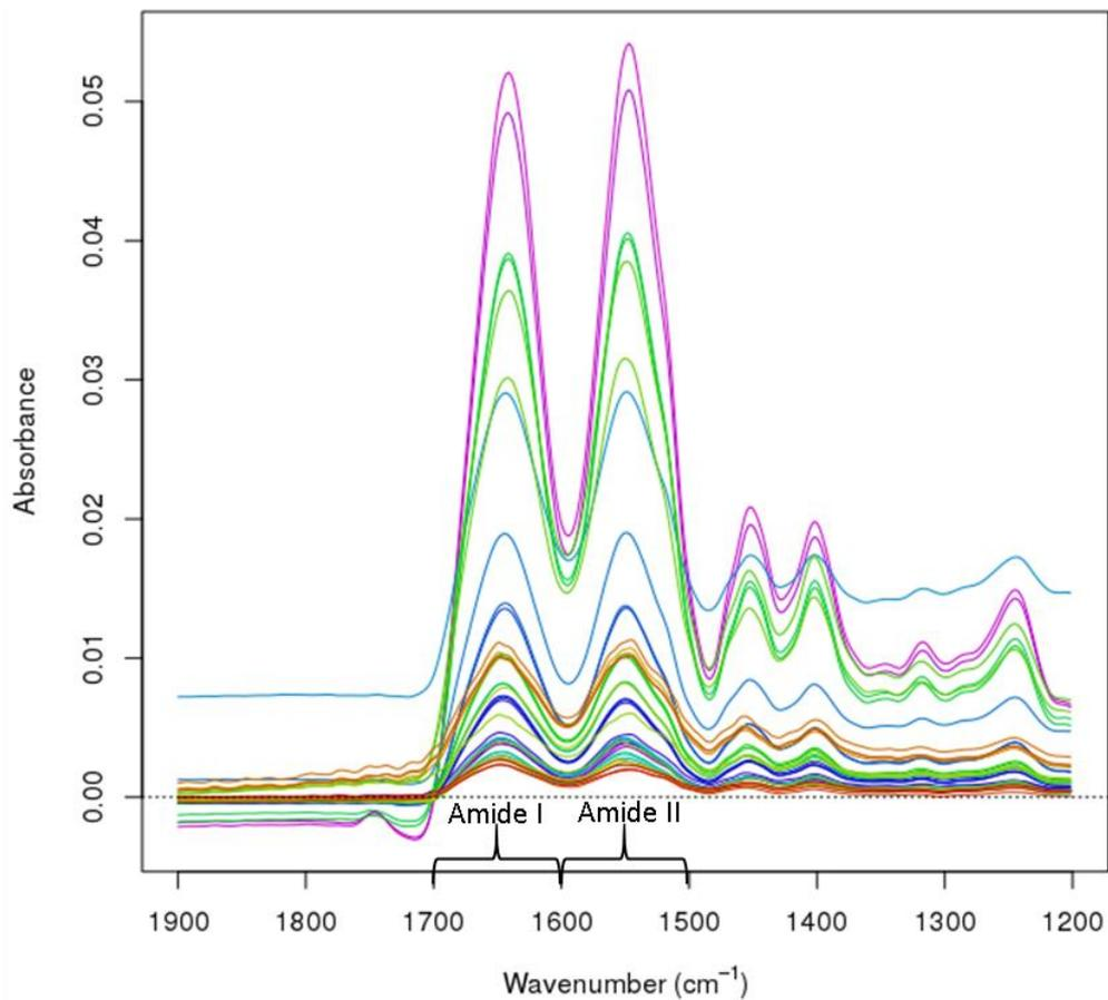
Figure 6. Raw spectra obtained through FTIP spectroscopy on casein, peptide and mixture stock solutions at  $50 \text{ g.kg}^{-1}$  and  $100 \text{ g.kg}^{-1}$ , as well as equilibrated samples at different concentrations.
