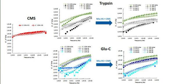
Fig.3 Frequency dependence of the elastic (G') and loss (G'') moduli for CMS and CMS + HS at 200 g.kg<sup>-1</sup> and pH 7.
