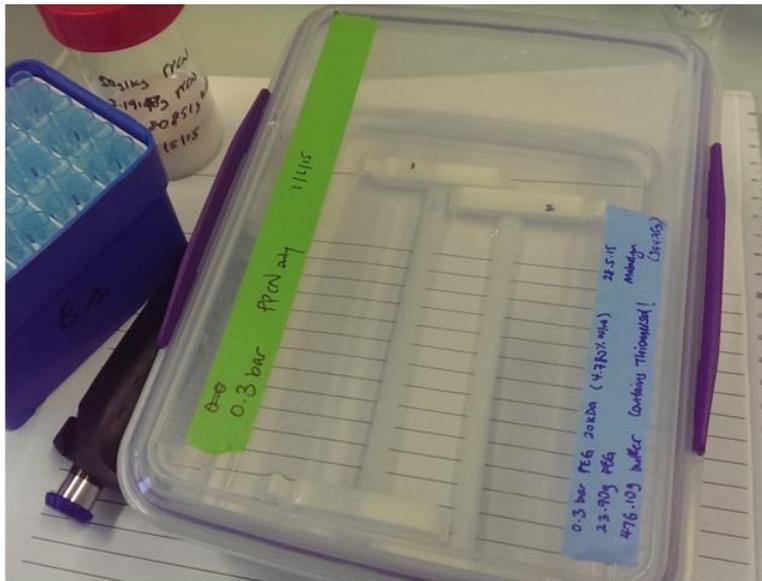
Figure 2. Set-up dialysis, with duplicate tubes filled with casein-peptide suspensions and placed in a sealed, transparent plastic box with PEG solution of required osmotic pressure.
