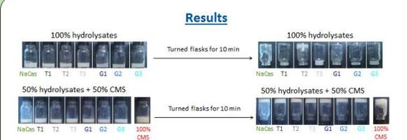
Fig.1 Gel formation by mixing HS and CMS at different ratio, at 200 g.kg<sup>-1</sup>, pH 7 and 20°C.
