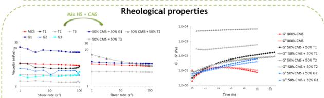
Fig. 3 Shear rate dependence of apparent viscosity for CMS, HS and mix CMS-HS at 100 g.kg<sup>-1</sup> and pH 7. Fig. 4 Time dependence of the elastic (G') and loss (G'') moduli for CMS and CMS + HS at 200 g.kg<sup>-1</sup> and pH 7.
