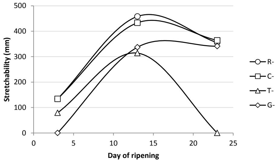
Fig. 4. Changes in stretchability during ripening of MMV cheese manufactured without NaCl (-) using ultrafiltrate retentate (R) as a control, and with 15 % (w/w) sodium caseinate (C), hydrolysate G (G) and hydrolysate T (T).
