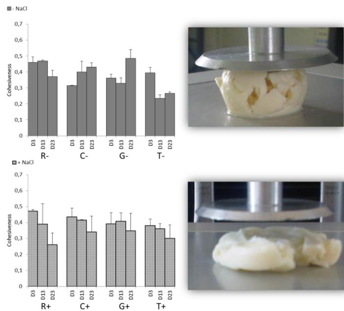
Fig. 5. Cohesiveness of cheeses at 3 (D3), 13 (D13) and 23 (D23) days of ripening. Cheeses are manufactured with ultrafiltrate retentate (R), used as a control, and with 15% (w/w) sodium caseinate (C), Trypsin hydrolysate (T) and Glu-C hydrolysate (G), with (+ in light grey) or without (- in dark grey) NaCl. The mean and SEM are represented. The photographs show the weak cohesiveness of the cheeses.
