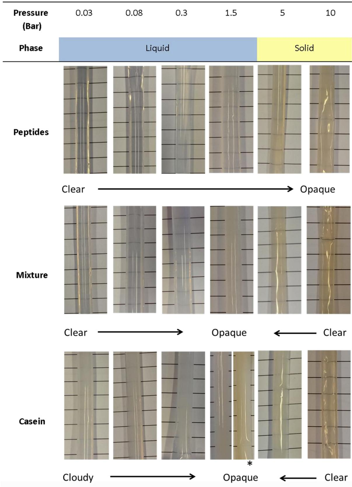
Figure 3. Visual observation of the peptide, mixture and casein suspensions at various pressure values inside the membrane 100-500 Da. \* Sample form duplicate trial for casein at 1.5 bar.
