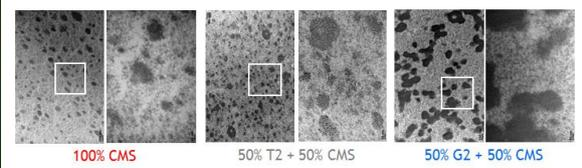
Fig.4 Electron micrograph of CMS, CMS + T2 and CMS + G2 at 200 g.kg<sup>-1</sup>, pH 7 and 20°C.
