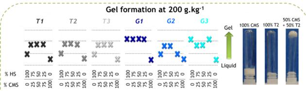
Fig. 1 Diagram of properties of CMS +/- HS at 200 g.kg<sup>-1</sup>, pH 7 and 20 °C. Fig. 2 Gel formation by mixing T2 and CMS at 200 g.kg<sup>-1</sup>, pH 7 and 20 °C.
