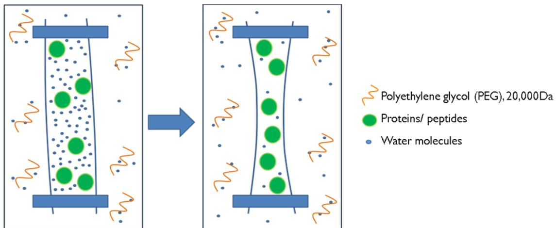
Figure 1. Water molecules from a protein-peptide solution is drawn out of the semi-permeable membrane, into a PEG solution of higher pressure.
