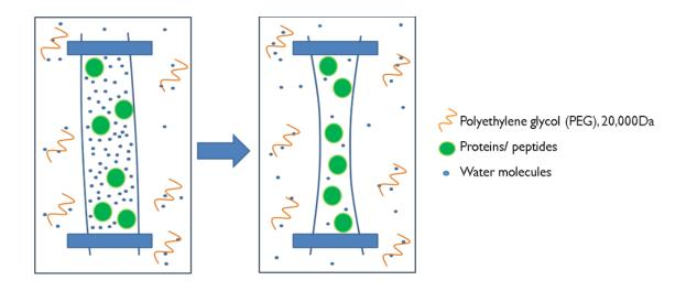
Figure 1. Water molecules from a protein-peptide solution is drawn out of the semi-permeable membrane, into a PEG solution of higher pressure.
