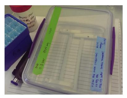
Figure 2. Set-up dialysis, with duplicate tubes filled with casein-peptide suspensions and placed is a sealed, transparent plastic box with PEG solution of required osmotic pressure.
