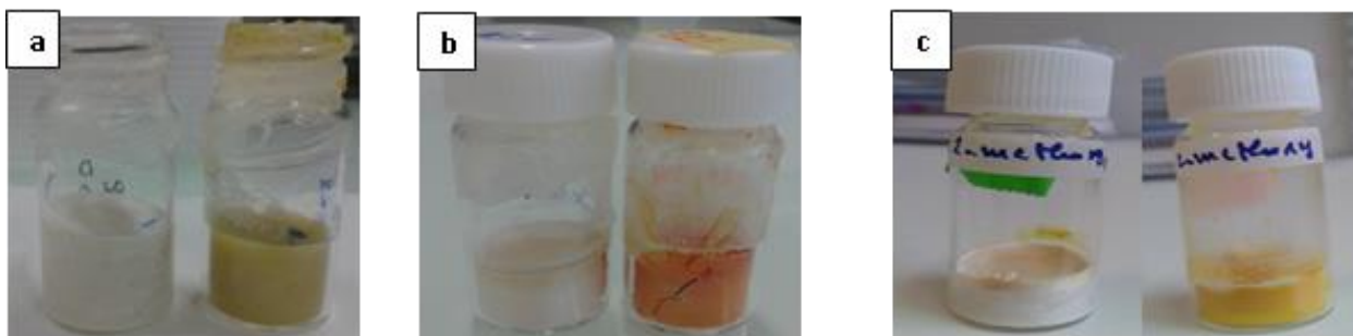
Figure III.S3 : Synthesized NIPs and IIPs with (a) DMSO, (b) ACN, and (c) 2-methoxyethanol In each picture, the NIP is on the left
