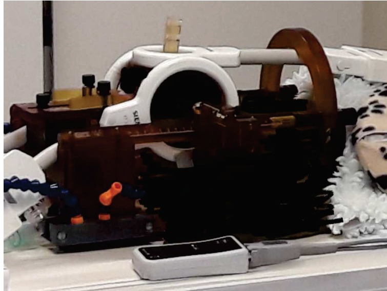
Figure 19: Setup for DTI acquisition with two L22 coils and one L7coil in anesthetized monkey.
