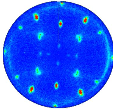
Figure 3.19 – In-plane pole figure at the fixed  $2\theta$  position of  $45^\circ$  of the  $\{10\bar{1}2\}$  planes of the intermetallic on a Ni 80 nm/InGaAs/InP sample after an  $350^\circ\text{C}$  RTA annealing. Corresponding stereographic projection is given in Figure 3.11b.
