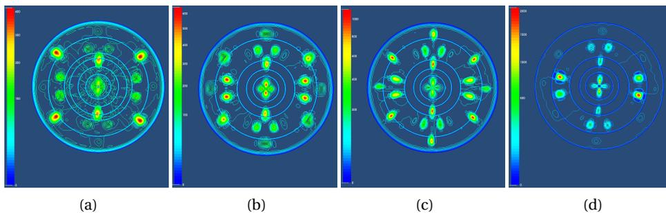
Figure 3.16 – Pole figure of the  $\{10\bar{1}1\}$  planes of the intermetallic hexagonal phase measured after the following annealings: (a) 300 °C, (b) 400 °C, (c) 450 °C, (d) 550 °C. The samples were measured using a Smartlab Rigaku diffractometer. Samples used are Ni(20 nm)/InGaAs/InP.
