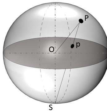
Figure 2.9 – Construction of a stereographic projection.
