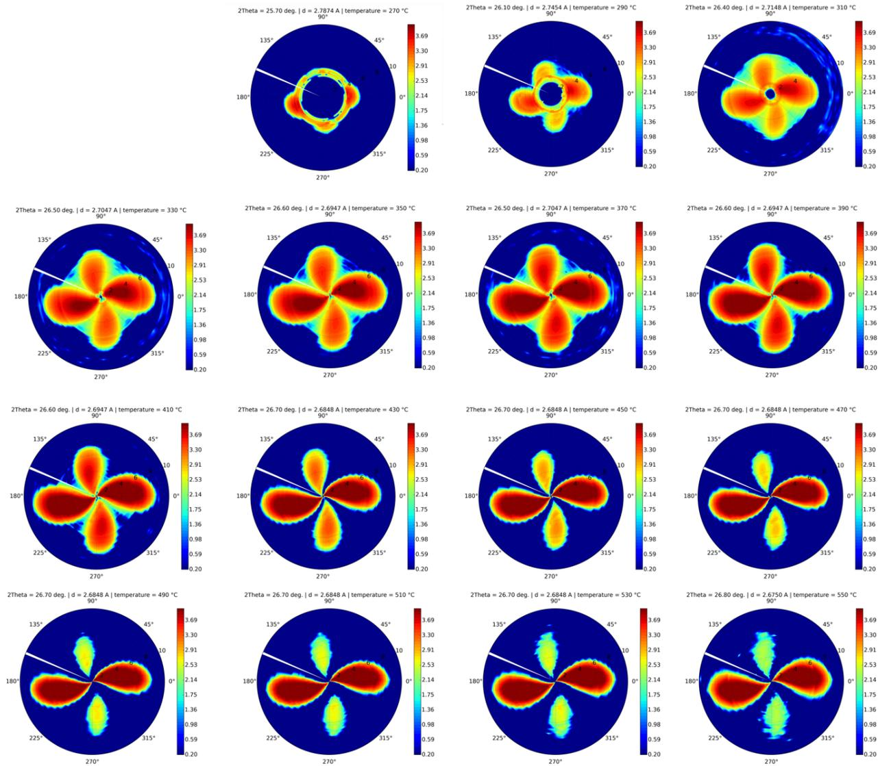
Figure 4.29 – Series of portion of the pole figures corresponding to the  $\{10\bar{1}1\}$  limited to  $\chi$  values between 0 and 10°. Each pole figure correspond to an annealing temperature starting from 270 °C and ending with 550 °C. The four poles in each pole figure correspond to the four  $\{10\bar{1}1\}$  planes that are located near the sample surface. The out-of plane region was not entirely accessible by measurement on the area detector for the first four pole figures.
