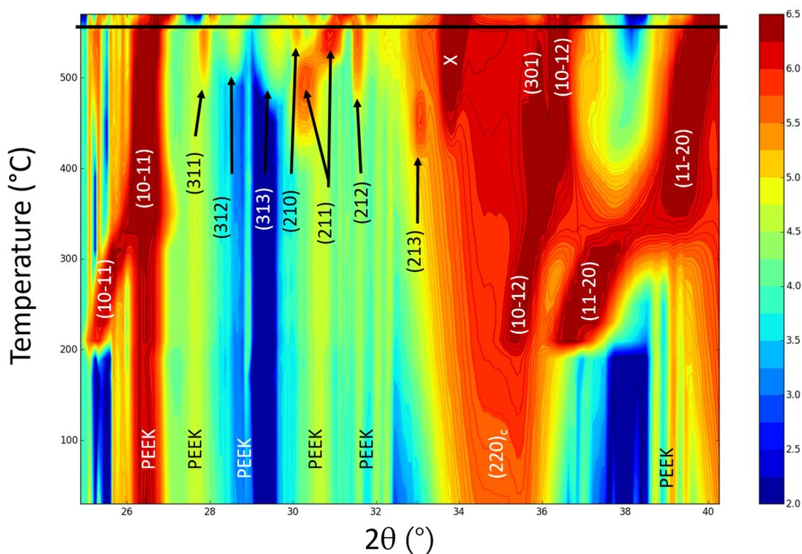
Figure 4.1 – Color map of the evolution of intensities according to  $2\theta$  angle and annealing temperature of the ramp for a Ni (20 nm)/InGaAs/InP sample. The bold black line at 550 °C denotes the measurement after slow cooling to room temperature.
