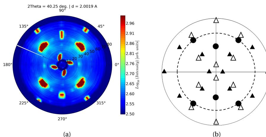
Figure 3.11 – (a) Pole figure of the  $\{10\bar{1}2\}$  planes of the intermetallic hexagonal phase measured after a 350 °C, (b) corresponding stereographic projection. The pole symbols are the same as defined in Table 3.1 and the dashed circle on stereographic projection represent the area that was actually measured. Samples used are Ni(20 nm)/InGaAs/InP.
