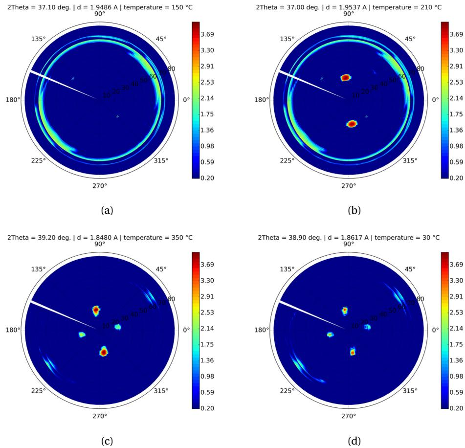
Figure 4.19 – Pole figures of the  $\{11\bar{2}0\}$  planes of the hexagonal lattice, measured at 10 keV at different ramp temperature (a) as-deposited (no intermetallic is formed yet), (b) at 250 °C, (c) at 350 °C and (d) at 30 °C after slow cooling to room temperature. The used sample is Ni(7 nm)/InGaAs/InP.
