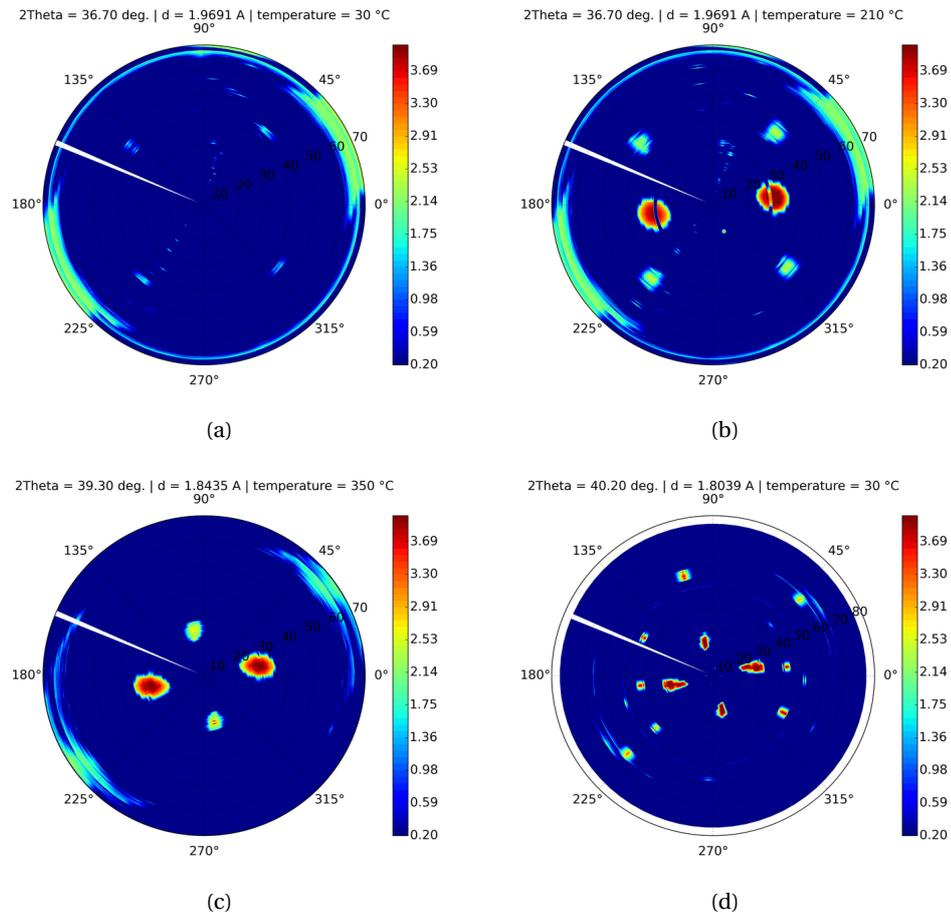
Figure 4.11 – Pole figures of the  $\{11\bar{2}0\}$  planes of the hexagonal lattice, measured at 10 keV at different ramp temperatures (a) as-deposited (no intermetallic is formed yet), (b) at  $250$  °C, (c) at  $350$  °C and (d) at  $30$  °C after slow cooling to room temperature. The used sample is Ni (20 nm)/InGaAs/InP.
