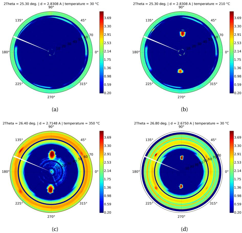
Figure 4.9 – Pole figures of the  $\{10\bar{1}1\}$  planes of the hexagonal lattice, measured at 10 keV at different ramp temperatures (a) as-deposited (no intermetallic is formed yet), (b) at 250 °C, (c) at 350 °C and (d) at 30 °C after slow cooling to room temperature. The used sample is Ni (20 nm)/InGaAs/InP.
