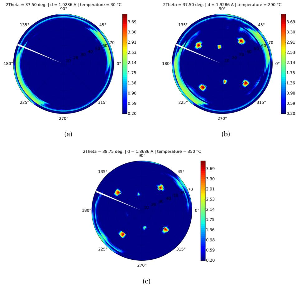
Figure 4.26 – Pole figures of the  $\{1\ 1\ \bar{2}\ 0\}$  planes of the hexagonal lattice, measured at 10 keV at different ramp temperature (a) as-deposited (no intermetallic is formed yet), (b) at 250 °C and (c) at 350 °C. Pole figure for the sample after cooling is not exploitable due to heavy PEEK diffraction overlapping. Sample used is Ni<sub>0.9</sub>Co<sub>0.1</sub> (20 nm)/InGaAs/InP.
