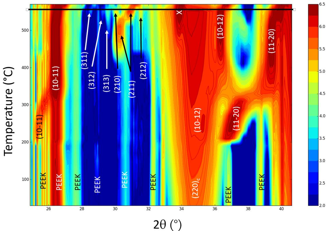
Figure 4.14 – Color map of the evolution of intensities according to  $2\theta$  angle and annealing temperature of the ramp for a Ni (7 nm)/InGaAs/InP sample. The bold black line at 550 °C denotes the measurement after slow cooling to room temperature. Sample used is Ni(7 nm)/InGaAs/InP.
