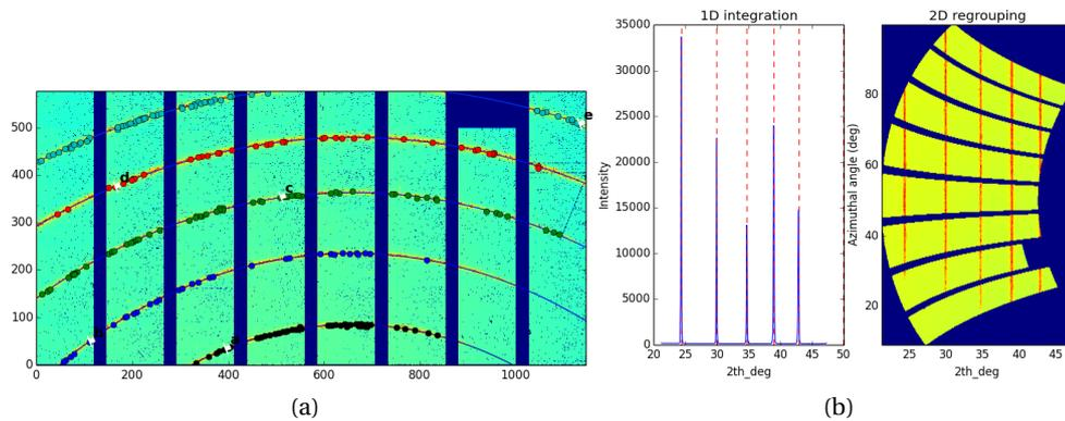
Figure 2.22 – (a) Powder diffraction image in pixel coordinates before calibration by PyFAI (b) Powder diffraction image and 1D integration after pixel to angular coordinates transformation.
