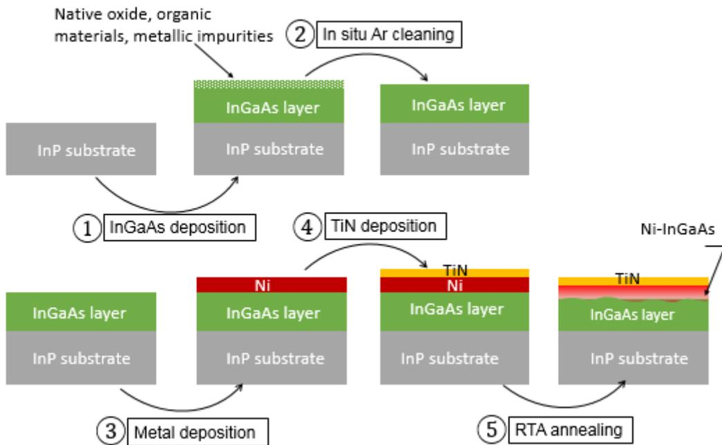
Figure 3.2 – Illustration of the different steps to produce the full sheet samples with reacted metal.
