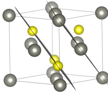
Figure 3.24 – The  $\{111\}$  planes in the InGaAs zinc-blende structure: alternatively planes containing only In or Ga (group III elements) and planes containing only As (group V elements). As is represented by big gray spheres while In and Ga are represented by small yellow spheres.
