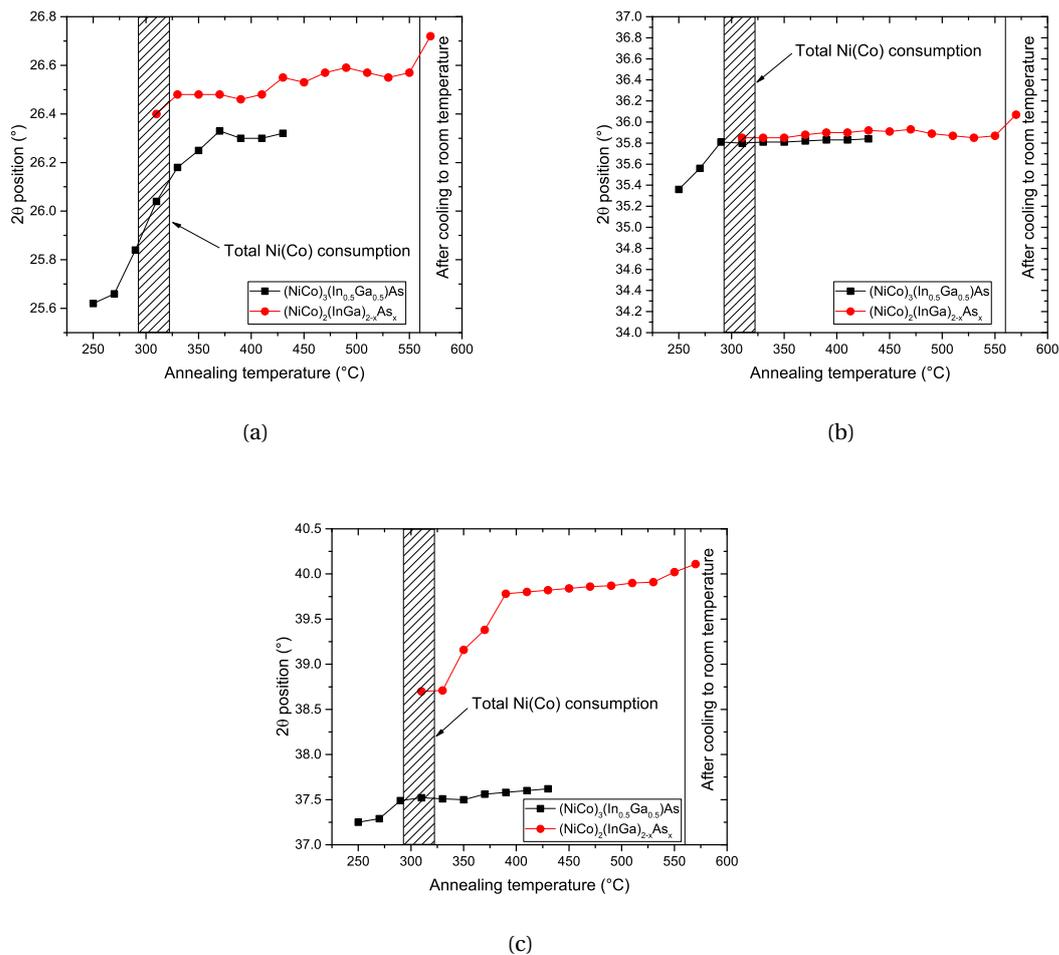
Figure 4.22 – Peak position according to the ramp annealing temperature of the (a)  $\{10\bar{1}1\}$ , (b)  $\{10\bar{1}2\}$  and (c)  $\{11\bar{2}0\}$  planes. Sample used is  $\text{Ni}_{0.9}\text{Co}_{0.1}$  (20 nm)/InGaAs/InP.
