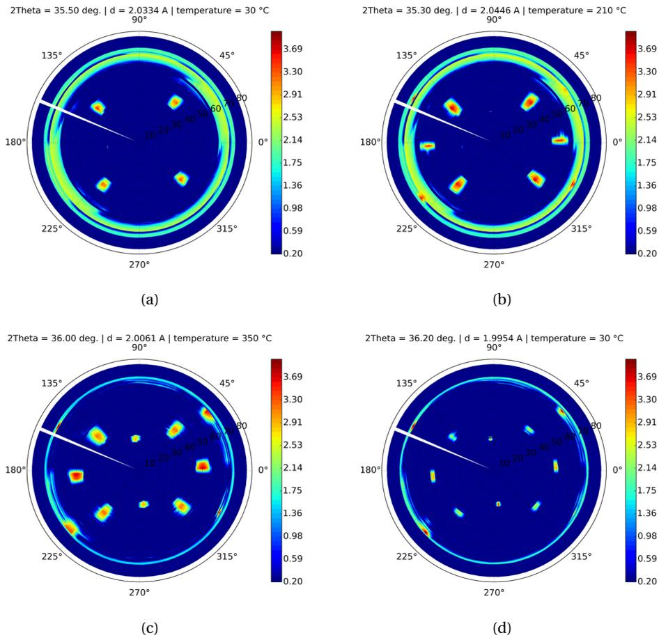
Figure 4.18 – Pole figures of the  $\{10\bar{1}2\}$  planes of the hexagonal lattice, measured at 10 keV at different ramp temperature (a) as-deposited (no intermetallic is formed yet), (b) at  $250$  °C, (c) at  $350$  °C and (d) at  $30$  °C after slow cooling to room temperature. The used sample is Ni(7 nm)/InGaAs/InP.
