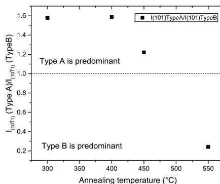
Figure 3.17 – Ratio of the relative intensities between  $I_{(10\bar{1}1)}$  of group A and  $I_{(10\bar{1}1)}$  of group B according to temperature.
