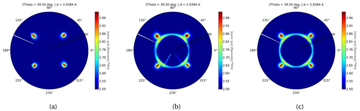
Figure 3.14 – (a) Pole figure at  $2\theta=39.5^\circ$  for a reference sample without metal deposition (InGaAs/InP), (b) pole figure of the  $\{111\}$  planes of the deposited NiCo for an as-deposited sample and (c) pole figure of the  $\{111\}$  planes of the deposited NiCo after annealing to 250 °C. Samples used are  $\text{Ni}_{0.9}\text{Co}_{0.1}$  (20 nm)/InGaAs/InP.
