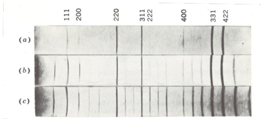
Figure 1.8 – Powder diffraction patterns of the superlattice Cu<sub>3</sub>Au (a) Disordered, (b) partially ordered, (c) highly ordered, (From [62]).
