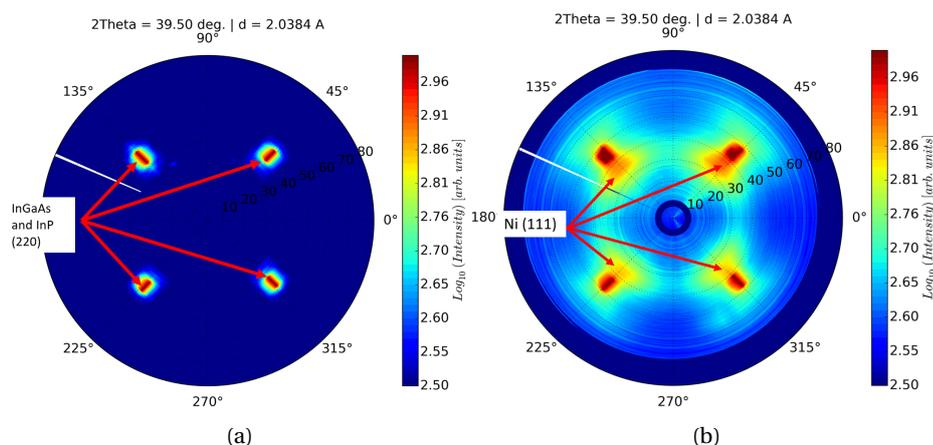
Figure 3.9 – (a) Pole figure at  $2\theta = 39.5^\circ$ , the eventual Ni {1 1 1} planes position at X-ray energy 10 keV for an InGaAs/InP sample (with no deposited metal), (b) Pole figure of the {1 1 1} planes of the deposited Ni on a sample annealed at 250 °C. Samples used are Ni(20 nm)/InGaAs/InP.
