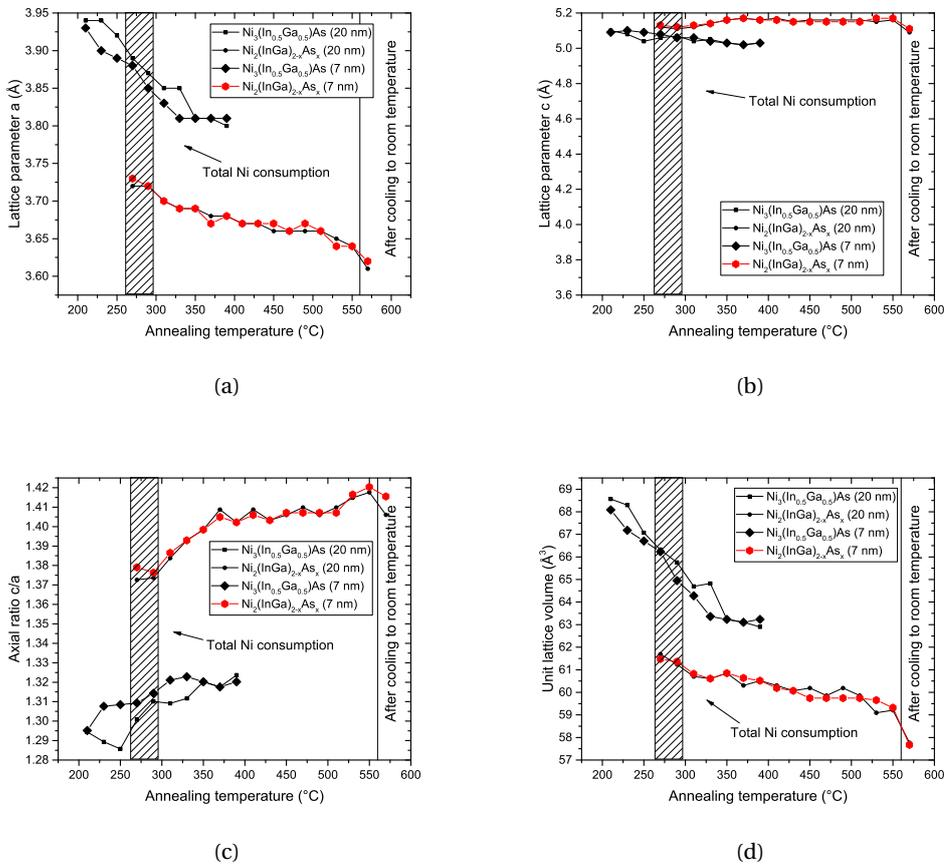
Figure 4.16 – Calculated parameters of the intermetallic hexagonal lattice (a)  $a$  lattice parameter, (b)  $c$  lattice parameter (c)  $c/a$  axial ratio and (d) volume of the hexagonal lattice. Sample used is Ni(7 nm)/InGaAs/InP.
