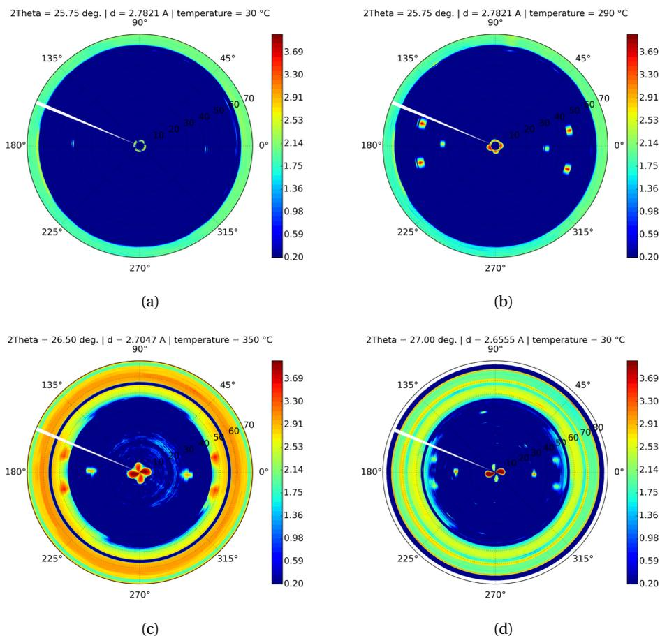
Figure 4.24 – Pole figures of the  $\{10\bar{1}1\}$  planes of the hexagonal lattice, measured at 10 keV at different ramp temperature (a) as-deposited (no intermetallic is formed yet), (b) at 250 °C, (c) at 350 °C and (d) at 30 °C after slow cooling to room temperature. Sample used is  $\text{Ni}_{0.9}\text{Co}_{0.1}$  (20 nm)/InGaAs/InP.
