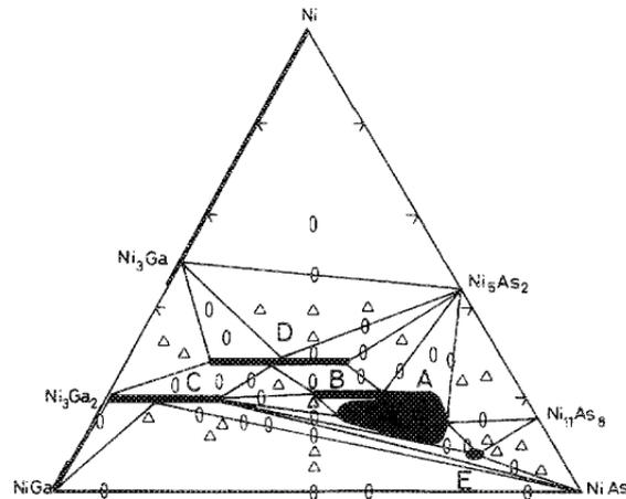
Figure 1.9 – Emphasized Ni-Ga-As diagram between the Ni<sub>3</sub>Ga-Ni<sub>5</sub>As<sub>2</sub> and NiGa-NiAs tie lines. The isothermal section of the solidus portion of the bulk Ni-Ga-As ternary diagram have features that are valid from 298 K up to the first eutectic point ( $T > 1073$  K) [23].
