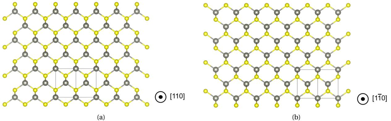
Figure 3.25 – A stack of InGaAs lattices projected along  $[110]$  in (a) and along the  $[\bar{1}10]$  direction in (b). As is represented by big gray spheres while In and Ga are represented by small yellow spheres. The unit lattice is marked by a rectangle on the figures.
