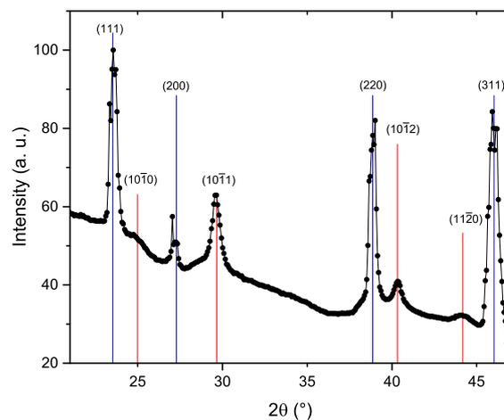
Figure 3.6 – X-Ray diffractogram of a sample after a 350 °C annealing. Red lines correspond to the intermetallic peak positions and blue lines correspond to InP/  $\text{In}_{0.53}\text{Ga}_{0.47}\text{As}$  peak position. X-Ray energy was set to 9 keV.
