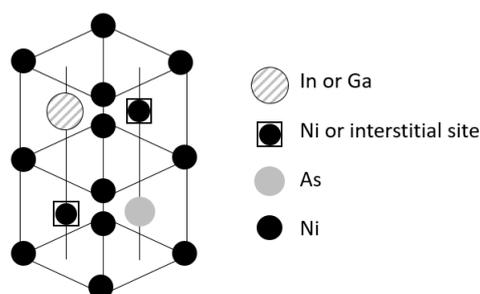
Figure 4.6 – Illustration of the unit cell of  $\text{Ni}_3\text{In}_{0.5}\text{Ga}_{0.5}\text{As}$ .
