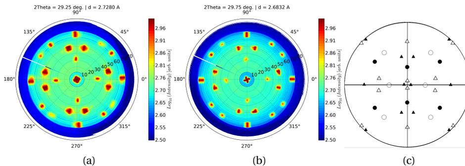
Figure 3.13 – (a) and (b), the pole figures of intermetallic  $\{10\bar{1}1\}$  planes after an RTA annealing of respectively 350 °C and 550 °C, (b) Corresponding stereographic projection. The as-deposited samples used are Ni(20 nm)/InGaAs/GaAs/Si.
