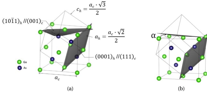
Figure 3.22 – (a) Transformation scheme of cubic unit cell of zinc blende-type structure in an hexagonal lattice with an ideal ratio of  $c/a = \sqrt{3}/\sqrt{2}$  (adapted from Lahav [64]), (b) Transformation scheme of cubic unit cell of zinc blende-type structure in an hexagonal lattice with a ratio of 1.4, the angle between the  $(001)_c$  and  $(10\bar{1}1)_h$  is denoted  $\alpha$ .
