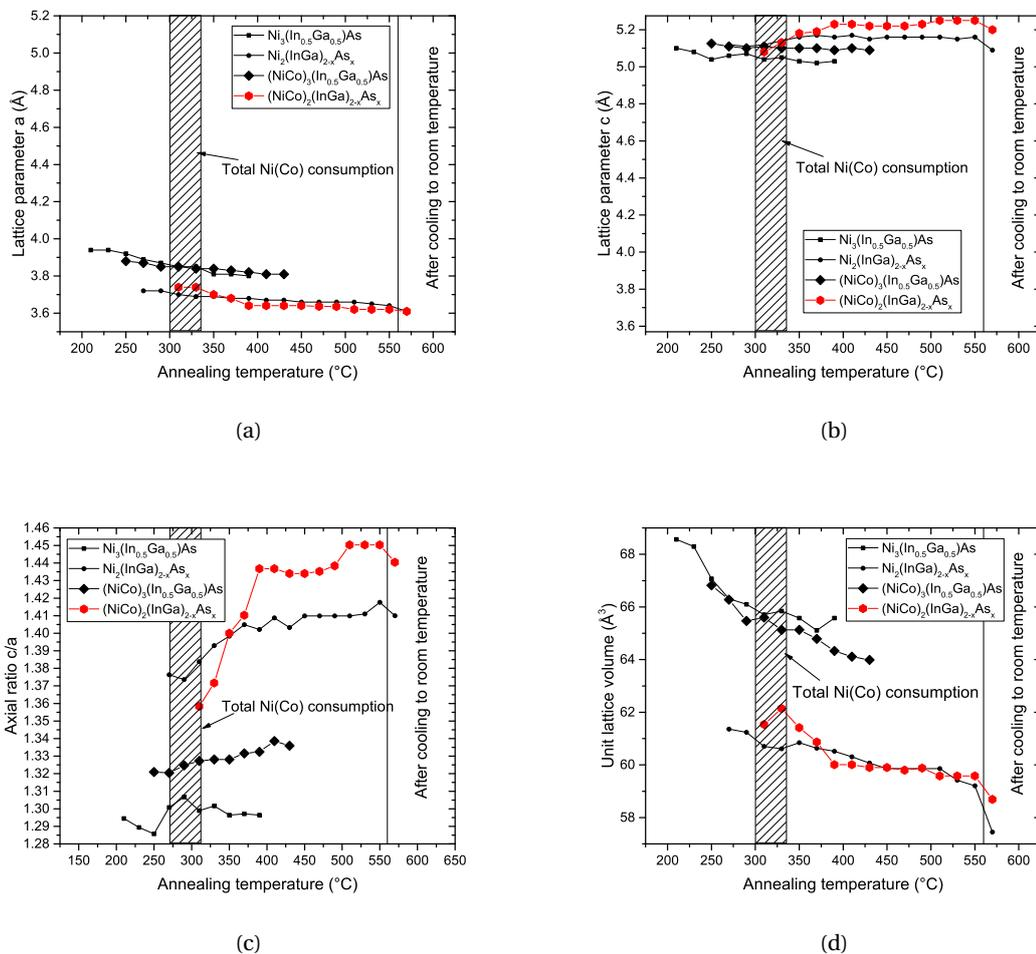
Figure 4.23 – Calculated parameters of the intermetallic hexagonal lattice (a) *a* lattice parameter, (b) *c* lattice parameter (c) *c/a* axial ratio and (d) volume of the hexagonal lattice. Sample used is Ni<sub>0.9</sub>Co<sub>0.1</sub>(20 nm)/InGaAs/InP.
