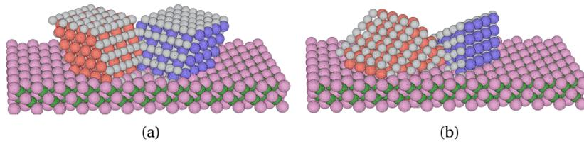
Figure 4.32 – Illustration of the orientations of (a) group A domains and (b) group B domains, against a zinc-blende structure.
