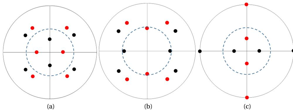
Figure 4.30 – Stereographic projections of group A oriented domains of (a)  $(10\bar{1}1)$ , (b)  $(10\bar{1}2)$  and (c)  $(11\bar{2}0)$  planes. The black poles belong to one azimuthal variant and the red poles belong to the second azimuthal variant.
