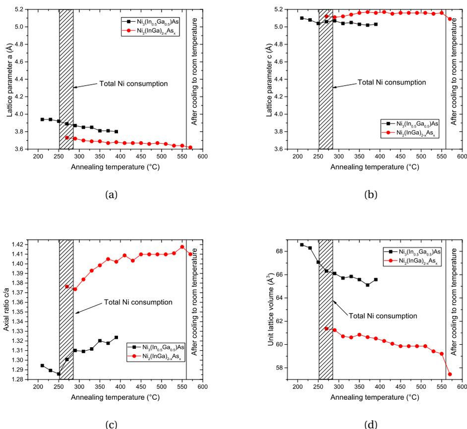
Figure 4.5 – Calculated parameters of the intermetallic hexagonal lattice (a)  $a$  lattice parameter, (b)  $c$  lattice parameter (c)  $c/a$  axial ratio and (d) volume of the hexagonal lattice. The used sample is Ni(20 nm)/InGaAs/InP.
