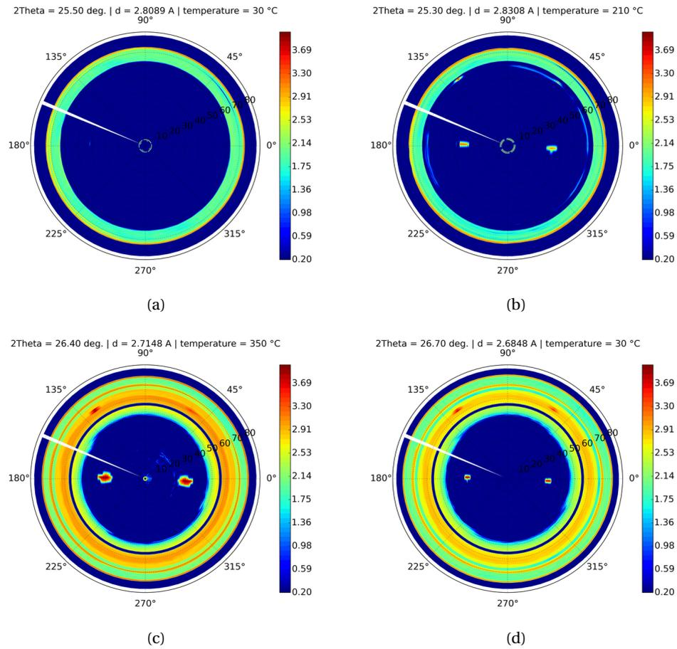
Figure 4.17 – Pole figures of the  $\{10\bar{1}1\}$  planes of the hexagonal lattice, measured at 10 keV at different ramp temperature (a) as-deposited (no intermetallic is formed yet), (b) at  $250$  °C, (c) at  $350$  °C and (d) at  $30$  °C after slow cooling to room temperature. The used sample is Ni(7 nm)/InGaAs/InP.
