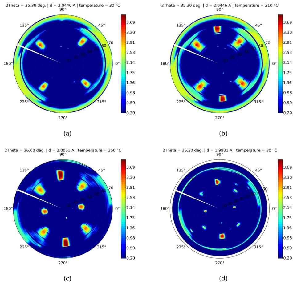
Figure 4.10 – Pole figures of the  $\{10\bar{1}2\}$  planes of the hexagonal lattice, measured at 10 keV at different ramp temperatures (a) as-deposited (no intermetallic is formed yet), (b) at 250 °C, (c) at 350 °C and (d) at 30 °C after slow cooling to room temperature. The used sample is Ni (20 nm)/InGaAs/InP.
