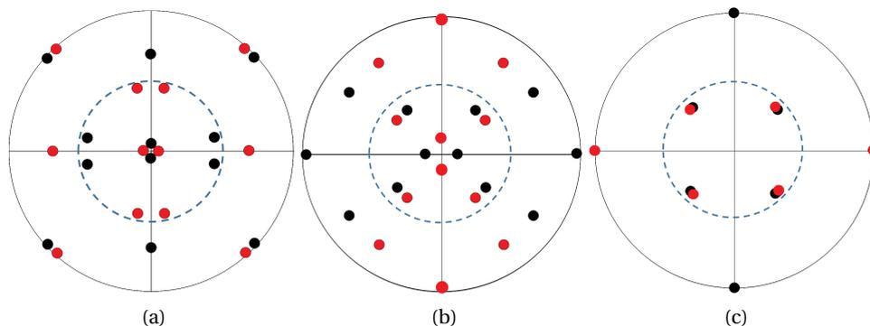
Figure 4.31 – Stereographic projections of group B oriented domains of (a)  $(10\bar{1}1)$ , (b)  $(10\bar{1}2)$  and (c)  $(11\bar{2}0)$  planes. The black poles belong to one azimuthal variant and the red poles belong to the second azimuthal variant.
