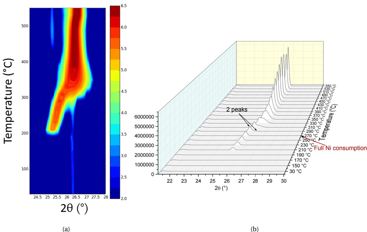
Figure 4.2 – (a) Color map of the evolution of intensities according to  $2\theta$  angle and annealing temperature of the ramp for the a uniquely integrated  $(10\bar{1}1)$  pole (situated at  $\chi=30^\circ$ ,  $\phi=90^\circ$  in Figure 4.9c). (b) 3D Waterfall view of the  $(10\bar{1}1)$  peak according to annealing temperature.
