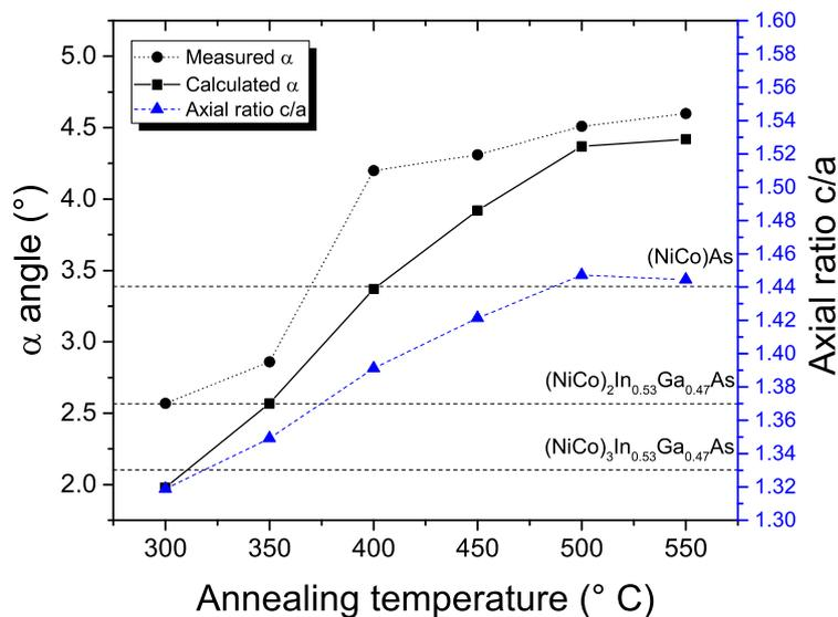
Figure 3.29 – Measured and calculated tilt angles  $\alpha$  and  $c/a$  ratio according to the annealing temperature for Ni<sub>0.9</sub>Co<sub>0.1</sub>/InGaAs/InP samples.
