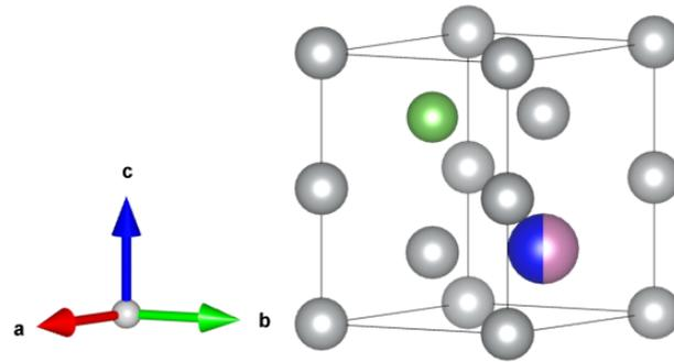
Figure 1.13 – Representation of a B8 Ni-InGaAs intermetallic with a stoichiometry of  $\text{Ni}_4\text{In}_{0.5}\text{Ga}_{0.5}\text{As}$ . Grey atoms correspond to Ni atoms, green atom correspond to As, blue atom correspond to In and pink atom correspond to Ga. In this example, the B8 structure is fully filled and there are 2 atoms on the metallic sub-cell.
