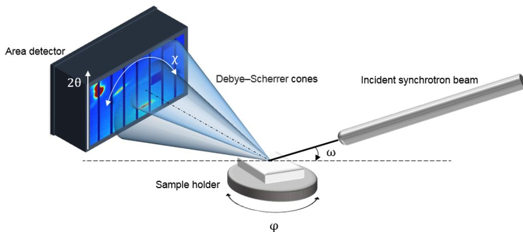
Figure 2.16 – Schematics of an are detector x-ray diffraction experiment on synchrotron. The area detectors has 2 degrees of liberty (lateral movement and a goniometer «  $2\theta$  » movement). The sample can rotate along  $\phi$ ,  $\chi$  and  $\omega$ .
