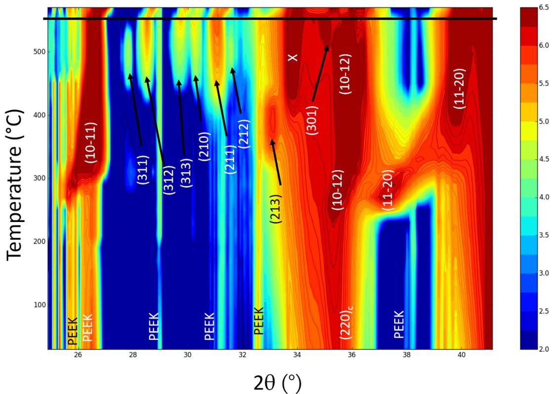
Figure 4.21 – Color map of the evolution of intensities according to  $2\theta$  angle and annealing temperature of the ramp for a Ni<sub>0.9</sub>Co<sub>0.1</sub>(20 nm)/InGaAs/InP sample. The bold black line at 550 °C denotes the measurement after slow cooling to room temperature.
