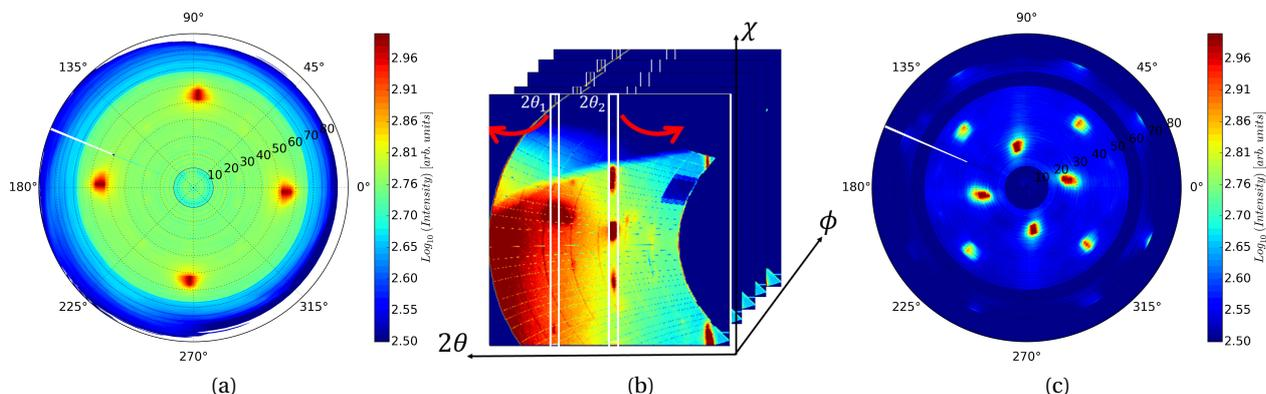
Figure 2.20 – Stitching process in the  $\chi$  direction (a) Pole figure at the  $2\theta_1$  position (b) Schematic example of a stack of diffraction images with two integration domains centered at  $2\theta_1$  and  $2\theta_2$  (c) Pole figure at the  $2\theta_2$  position.
