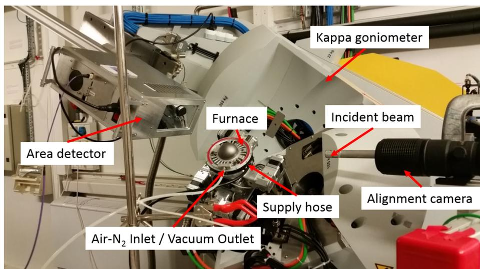
Figure 2.21 – Picture of the in-situ experiment on the D2AM beam-line. The sample is covered by a graphite dome.
