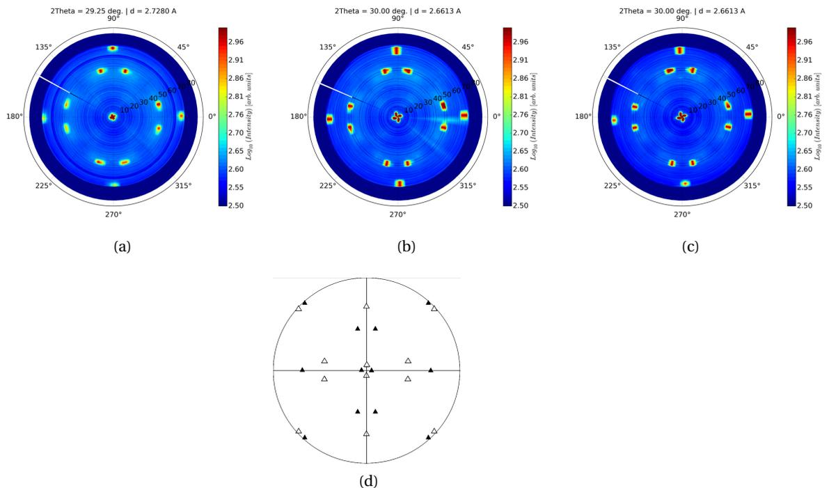
Figure 3.15 – Pole figures of the intermetallic  $\{10\bar{1}1\}$  planes after an RTA annealing of (a) 350 °C, (b) 450 °C, (c) 550 °C and (d) stereographic representation of the pole figures. Samples used are  $\text{Ni}_{0.9}\text{Co}_{0.1}$  (20 nm)/InGaAs/InP.
