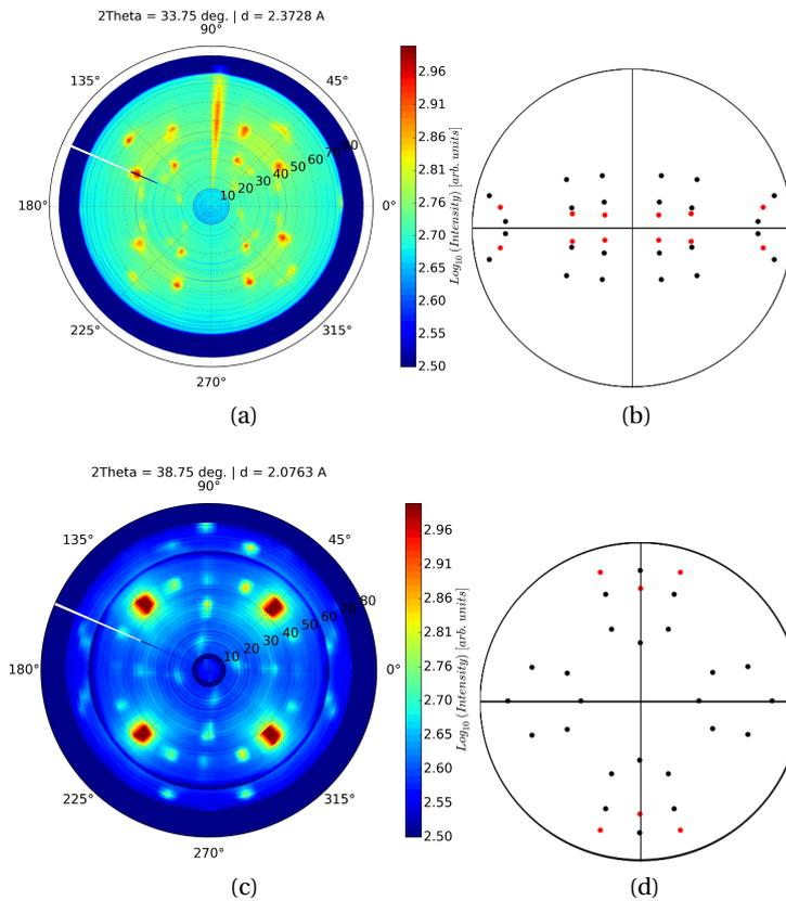
Figure 3.31 – Pole figures of respectively: (a)  $\{3\bar{1}2\}$  planes and (c)  $\{10\bar{1}7\}$  planes, and respectively their corresponding stereographic projections: (b) for  $\{3\bar{1}2\}$  planes and (d) for  $\{10\bar{1}7\}$  planes. Extra poles on (c) correspond to nearby diffraction peaks from substrate and main intermetallic. Group A variants are represented by red poles and group B variants are represented by black poles.
