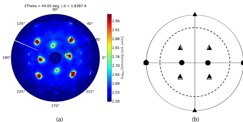
Figure 3.12 – (a) Pole figure of the  $\{11\bar{2}0\}$  planes of the intermetallic hexagonal phase measured after a 350 °C, (b) Corresponding stereographic projection. Extra poles on the pole figure correspond to the poles measured from the nearby  $\{311\}$  planes of the substrate. The pole symbols are the same as defined in Table 3.1 and the dashed circle on stereographic projection represent the area that was actually measured. Samples used are Ni(20 nm)/InGaAs/InP
