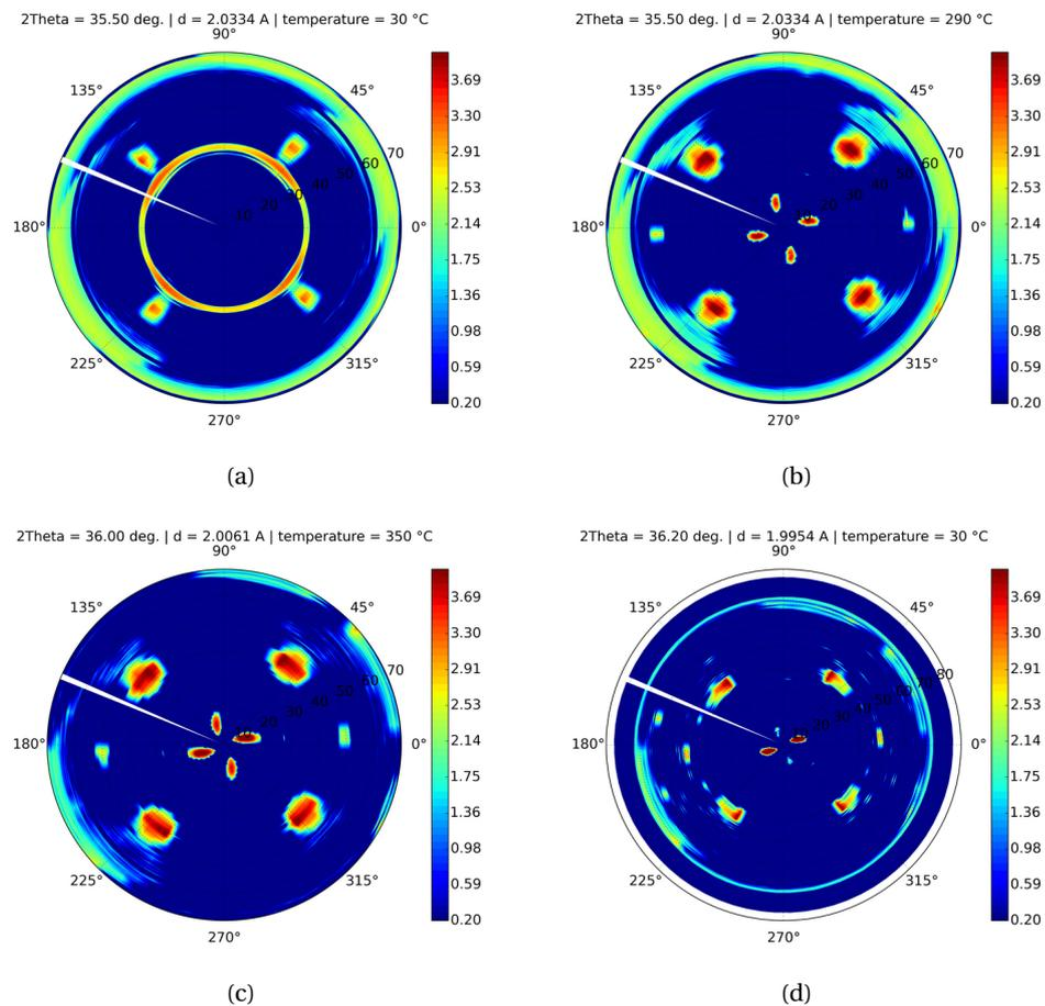
Figure 4.25 – Pole figures of the  $\{10\bar{1}2\}$  planes of the hexagonal lattice, measured at 10 keV at different ramp temperature (a) as-deposited (no intermetallic is formed yet), (b) at 250 °C, (c) at 350 °C and (d) at 30 °C after slow cooling to room temperature. Sample used is Ni<sub>0.9</sub>Co<sub>0.1</sub>(20 nm)/InGaAs/InP. The ring in as-deposited (a) pole figure shows fiber texture of deposited NiCo.
