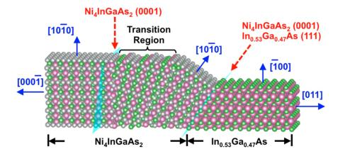
Figure 1.12 – Orientation of the hexagonal intermetallic as observed by Chen et al. [80] in an InGaAs Fin.
