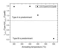
Figure 3.17 – Ratio of the relative intensities between  $I_{(10\overline{1}1)}$  of group A and  $I_{(10\overline{1}1)}$  of group B according to temperature.
