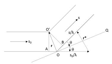
Figure 2.2 – O and O' are the point scatterers. s and  $s_0$  are unit vectors. Therefore AO =  $-r \cdot s_0$ , BO =  $r \cdot s$
