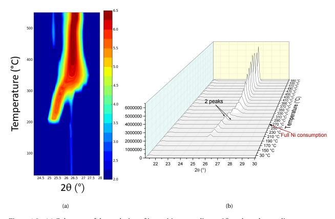
Figure 4.2 – (a) Color map of the evolution of intensities according to  $2\theta$  angle and annealing temperature of the ramp for the a uniquely integrated ( $10\overline{1}1$ ) pole (situated at  $\chi=30^\circ$ ,  $\phi=90^\circ$  in Figure 4.9c). (b) 3D Waterfall view of the ( $10\overline{1}1$ ) peak according to annealing temperature.
