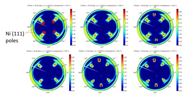
Figure 4.8 – Pole figure corresponding to the deposited Ni (111) plane position at several annealing temperatures from 170 to 270 °C. Ni poles are marked on the first pole figure (top-left). The remaining poles correspond to either the (220) planes of the substrate or to the intermetallic  $\{10\overline{1}2\}$  peaks.
