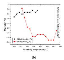
Figure 4.27 – Calculated mismatch between the intermetallic and the substrate considering an axiotaxial alignment for (a) Group A domains and (b) Group B domains.
