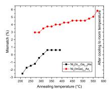
Figure 4.20 – Calculated mismatch between the intermetallic and the substrate considering an axiotaxial alignment for Group A domains. The used sample is Ni(7 nm)/InGaAs/InP.
