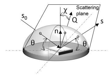
Figure 2.8 –  $\chi$  tilt defined in the sample referential. In practice, the scattering vector  $\mathbf{Q}$  is brought to diffraction conditions by rotating the sample by a  $\chi$  angle.
