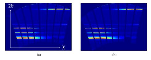
Figure 2.24 – Two diffraction images at the same  $\phi \delta$  and  $\chi$  position at: (a)  $v = 0^{\circ}$  and (b)  $v = 2^{\circ}$ .
