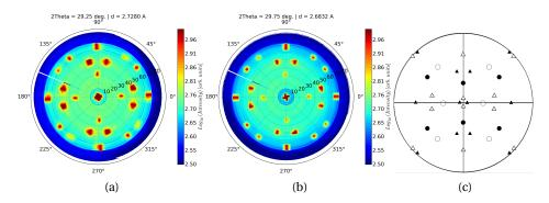
Figure 3.13 – (a) and (b), the pole figures of intermetallic  $\{10\overline{1}1\}$  planes after an RTA annealing of respectively 350 °C and 550 °C, (b) Corresponding stereographic projection. The as-deposited samples used are Ni(20 nm)/InGaAs/GaAs/Si.
