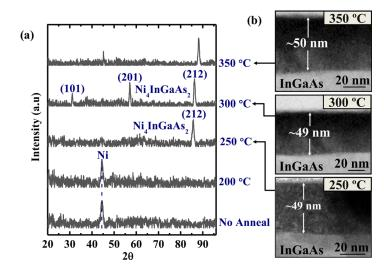
Figure 1.14 – (a) XRD general area detector diffraction system(GADDS) integrated diffraction intensity as a function of  $2\theta$ . (b) TEM images showing the thickness of 250, 300, and 350 °C formed films [78].
