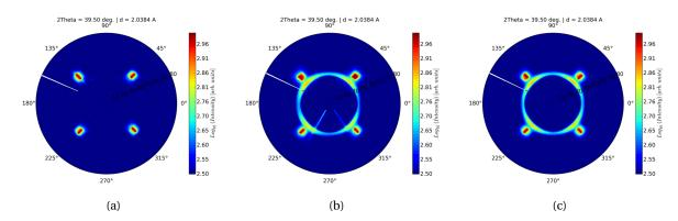
Figure 3.14 – (a) Pole figure at  $2\theta$ =39.5° for a reference sample without metal deposition (InGaAs/InP), (b) pole figure of the {111} planes of the deposited NiCo for an as-deposited sample and (c) pole figure of the {111} planes of the deposited NiCo after annealing to 250 °C. Samples used are Ni<sub>0.9</sub>Co<sub>0.1</sub>(20 nm)/InGaAs/InP.
