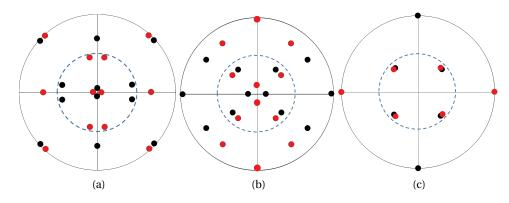
Figure 4.31 – Stereographic projections of group B oriented domains of (a)  $(10\overline{1}1)$ , (b)  $(10\overline{1}2)$  and (c)  $(11\overline{2}0)$  planes. The black poles belong to one azimuthal variant and the red poles belong to the second azimuthal variant.
