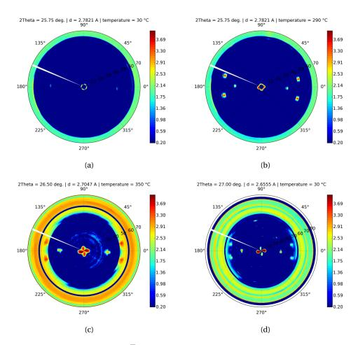
Figure 4.24 – Pole figures of the  $\{10\overline{1}1\}$  planes of the hexagonal lattice, measured at 10 keV at different ramp temperature (a) as-deposited (no intermetallic is formed yet), (b) at 250 °C, (c) at 350 °C and (d) at 30 °C after slow cooling to room temperature. Sample used is Ni<sub>0.9</sub>Co<sub>0.1</sub>(20 nm)/InGaAs/InP.
