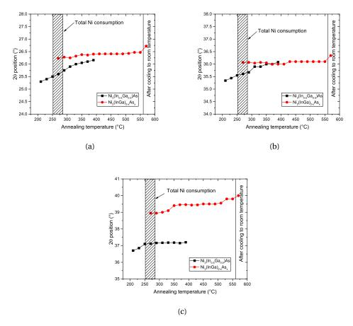
Figure 4.15 – Peak position according to the ramp annealing temperature of the (a)  $(10\overline{1}1)$ , (b)  $(10\overline{1}2)$  and (c)  $(11\overline{2}0)$  planes. Sample used is Ni(7 nm)/InGaAs/InP.
