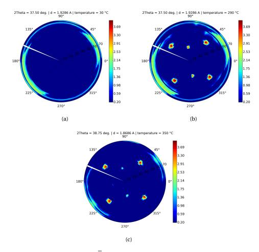
Figure 4.26 – Pole figures of the  $\{1\,1\,\overline{2}\,0\}$  planes of the hexagonal lattice, measured at 10 keV at different ramp temperature (a) as-deposited (no intermetallic is formed yet), (b) at 250 °C and (c) at 350 °C. Pole figure for the sample after cooling is not exploitable due to heavy PEEK diffraction overlapping. Sample used is Ni<sub>0.9</sub>Co<sub>0.1</sub>(20 nm)/InGaAs/InP.
