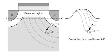
Figure 1 – Illustration of the punch-though phenomena in the case of a blocked NMOS.
