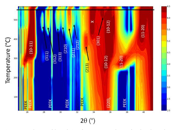
Figure 4.21 – Color map of the evolution of intensities according to  $2\theta$  angle and annealing temperature of the ramp for a Ni<sub>0.9</sub>Co<sub>0.1</sub>(20 nm)/InGaAs/InP sample. The bold black line at 550 °C denotes the measurement after slow cooling to room temperature.
