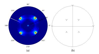
Figure 2.11 - (a) Pole Figure of  $\{1\,1\,0\}$  planes of a cubic lattice and (b) corresponding stereographic simulation on Carine Crystallography.
