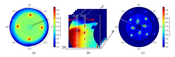
Figure 2.20 – Stitching process in the  $\chi$  direction (a) Pole figure at the  $2\theta_1$  position (b) Schematic example of a stack of diffraction images with two integration domains centered at  $2\theta_1$  and  $2\theta_2$  (c) Pole figure at the  $2\theta_2$  position.
