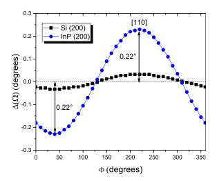
Figure 3.4 –  $\Delta(\Omega)$  evolution of the (200) peak position of the (200) planes for Si (squared black) and InP (dotted blue) according to  $\Phi$ .
