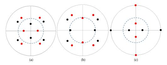
Figure 4.30 – Stereographic projections of group A oriented domains of (a)  $(10\overline{1}1)$ , (b)  $(10\overline{1}2)$  and (c)  $(11\overline{2}0)$  planes. The black poles belong to one azimuthal variant and the red poles belong to the second azimuthal variant.
