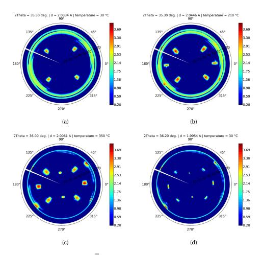
Figure 4.18 – Pole figures of the  $\{10\overline{1}2\}$  planes of the hexagonal lattice, measured at 10 keV at different ramp temperature (a) as-deposited (no intermetallic is formed yet), (b) at 250 °C, (c) at 350 °C and (d) at 30 °C after slow cooling to room temperature. The used sample is Ni(7 nm)/InGaAs/InP.
