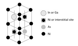
Figure 4.6 – Illustration of the unit cell of Ni<sub>3</sub>In<sub>0.5</sub>Ga<sub>0.5</sub>As.
