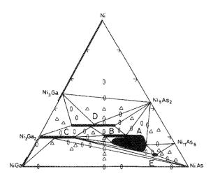
Figure 1.9 – Emphasized Ni-Ga-As diagram between the  $Ni_3Ga-Ni_5As_2$  and NiGa-NiAs tie lines. The isothermal section of the solidus portion of the bulk Ni-Ga-As ternary diagram have features that are valid from 298 K up to the first eutectic point (T > 1073 K) [23].
