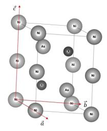
Figure 3.7 – Reduced lattice of the NiAs hexagonal structure. Atom position marked by X correspond to (2*d*) sites [67].
