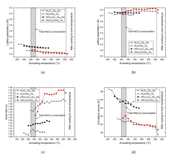
Figure 4.23 – Calculated parameters of the intermetallic hexagonal lattice (a) a lattice parameter, (b) c lattice parameter (c) c/a axial ratio and (d) volume of the hexagonal lattice. Sample used is Ni<sub>0.9</sub>Co<sub>0.1</sub>(20 nm)/InGaAs/InP.
