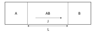
Figure 1.2 – Schematic presentation of the AB phase growth between the pure elements A and B by the diffusion of A atoms.
