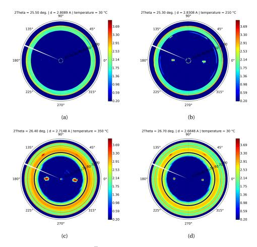
Figure 4.17 – Pole figures of the  $\{10\overline{1}1\}$  planes of the hexagonal lattice, measured at 10 keV at different ramp temperature (a) as-deposited (no intermetallic is formed yet), (b) at 250 °C, (c) at 350 °C and (d) at 30 °C after slow cooling to room temperature. The used sample is Ni(7 nm)/InGaAs/InP.
