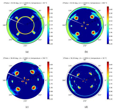
Figure 4.25 – Pole figures of the  $\{10\overline{1}2\}$  planes of the hexagonal lattice, measured at 10 keV at different ramp temperature (a) as-deposited (no intermetallic is formed yet), (b) at 250 °C, (c) at 350 °C and (d) at 30 °C after slow cooling to room temperature. Sample used is Ni<sub>0.9</sub>Co<sub>0.1</sub>(20 nm)/InGaAs/InP. The ring in as-deposited (a) pole figure shows fiber texture of deposited NiCo.
