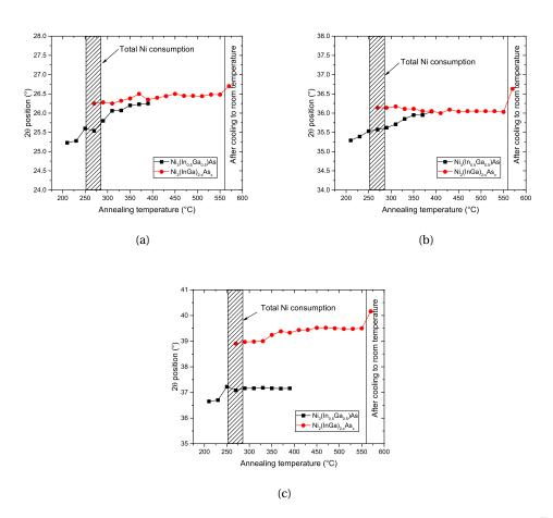
Figure 4.4 – Peak position according to the ramp annealing temperature of the (a)  $(10\overline{1}1)$ , (b)  $(10\overline{1}2)$  and (c)  $(11\overline{2}0)$  planes. The used sample is Ni(20 nm)/InGaAs/InP.
