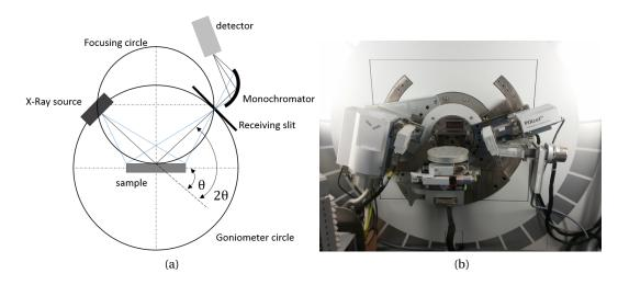
Figure 2.4 – Two-circle powder diffractometer: (a) Schematics of two-circle diffractometer, (b) picture of the PANalytical Empyrean goniometer.
