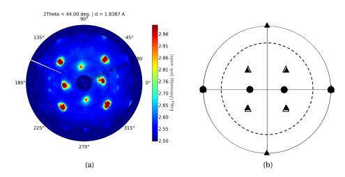
Figure 3.12 – (a) Pole figure of the  $\{1\,1\,\overline{2}\,0\}$  planes of the intermetallic hexagonal phase measured after a 350 °C, (b) Corresponding stereographic projection. Extra poles on the pole figure correspond to the poles measured from the nearby  $\{3\,1\,1\}$  planes of the substrate. The pole symbols are the same as defined in Table 3.1 and the dashed circle on stereographic projection represent the area that was actually measured. Samples used are Ni(20 nm)/InGaAs/InP
