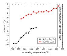
Figure 4.12 – Calculated mismatch between the intermetallics and the substrate considering an axiotaxial alignment for Group A domains.
