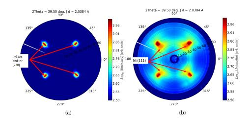
Figure 3.9 – (a) Pole figure at  $2\theta$  = 39.5°, the eventual Ni {111} planes position at X-ray energy 10 keV for an InGaAs/InP sample (with no deposited metal), (b) Pole figure of the {111} planes of the deposited Ni on a sample annealed at 250 °C. Samples used are Ni(20 nm)/InGaAs/InP.
