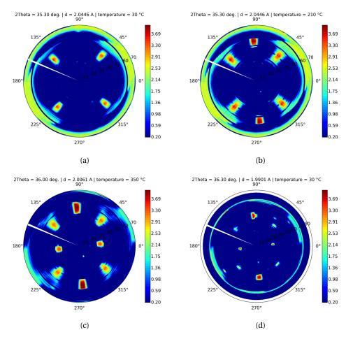
Figure 4.10 – Pole figures of the  $\{10\overline{1}2\}$  planes of the hexagonal lattice, measured at 10 keV at different ramp temperatures (a) as-deposited (no intermetallic is formed yet), (b) at 250 °C, (c) at 350 °C and (d) at 30 °C after slow cooling to room temperature. The used sample is Ni (20 nm)/InGaAs/InP.
