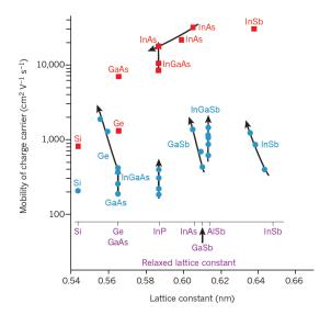
Figure 2 – Electron and hole mobility of group III–V compound semiconductors. The highest room-temperature mobility of electrons (red) and holes (blue) in inversion layers and quantum wells is shown as a function of the actual semiconductor lattice parameter [5].
