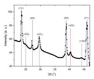
Figure 3.6 – X-Ray diffractogram of a sample after a 350 °C annealing. Red lines correspond to the intermetallic peak positions and blue lines correspond to InP/  $In_{0.53}Ga_{0.47}As$  peak position. X-Ray energy was set to 9 keV.
