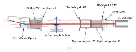
Figure 2.12 – 4-circles configuration of the smartlab: (a) Picture of the Smartlab 4-circles configuration, (b) Schematics of the Smartlab optics.
