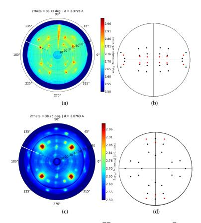
Figure 3.31 – Pole figures of respectively: (a)  $\{3\overline{12}1\}$  planes and (c)  $\{10\overline{17}\}$  planes, and respectively their corresponding stereographic projections: (b) for  $\{3\overline{12}1\}$  planes and (d) for  $\{10\overline{17}\}$  planes. Extra poles on (c) correspond to nearby diffraction peaks from substrate and main intermetallic. Group A variants are represented by red poles and group B variants are represented by black poles.
