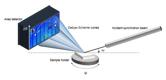
Figure 2.16 – Schematics of an are detector x-ray diffraction experiment on synchrotron. The area detectors has 2 degrees of liberty (lateral movement and a goniometer «  $2\theta$  » movement). The sample can rotate along  $\phi$ ,  $\chi$  and  $\omega$ .
