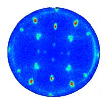
Figure 3.19 – In-plane pole figure at the fixed  $2\theta$  position of 45 ° of the  $\{10\overline{1}2\}$  planes of the intermetallic on a Ni 80 nm/InGaAs/InP sample after an 350 °C RTA annealing. Corresponding stereographic projection is given in Figure 3.11b.
