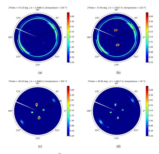
Figure 4.19 – Pole figures of the  $\{1\,1\,\overline{2}\,0\}$  planes of the hexagonal lattice, measured at 10 keV at different ramp temperature (a) as-deposited (no intermetallic is formed yet), (b) at 250 °C, (c) at 350 °C and (d) at 30 °C after slow cooling to room temperature. The used sample is Ni(7 nm)/InGaAs/InP.
