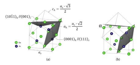
Figure 3.22 – (a) Transformation scheme of cubic unit cell of zinc blende-type structure in an hexagonal lattice with an ideal ratio of  $c/a = \sqrt{3}\sqrt{2}$  (adapted from Lahav [64]), (b) Transformation scheme of cubic unit cell of zinc blende-type structure in an hexagonal lattice with a ratio of 1.4, the angle between the  $(001)_c$  and  $(10\overline{1}1)_h$  is denoted  $\alpha$ .
