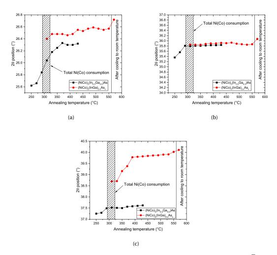
Figure 4.22 – Peak position according to the ramp annealing temperature of the (a)  $(10\overline{1}1)$ , (b)  $(10\overline{1}2)$  and (c)  $(11\overline{2}0)$  planes. Sample used is Ni<sub>0.9</sub>Co<sub>0.1</sub>(20 nm)/InGaAs/InP.
