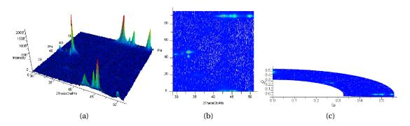
Figure 2.14 – Example of an in plane RSM measurement: (a) Topographical view, (b) flat view and (c) reciprocal space coordinates view.
