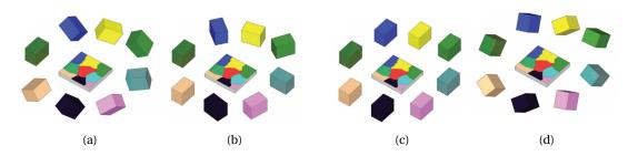
Figure 1.5 – Distribution of the crystallographic orientations: (a) random texture, (b) fiber texture, (c) epitaxial texture, (d) axiotaxial texture (adapted from [59]).
