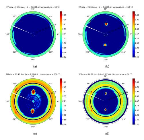
Figure 4.9 – Pole figures of the  $\{1\,0\,\overline{1}\,1\}$  planes of the hexagonal lattice, measured at 10 keV at different ramp temperatures (a) as-deposited (no intermetallic is formed yet), (b) at 250 °C, (c) at 350 °C and (d) at 30 °C after slow cooling to room temperature. The used sample is Ni (20 nm)/InGaAs/InP.
