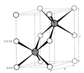
Figure 1.7 – The hexagonal NiAs, B8<sub>1</sub> structure. Non-filled circles represent metallic atoms and hatched circles represent the metalloid/post-transition metal atoms [60].
