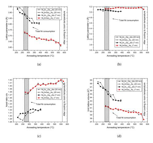
Figure 4.16 – Calculated parameters of the intermetallic hexagonal lattice (a) a lattice parameter, (b) c lattice parameter (c) c/a axial ratio and (d) volume of the hexagonal lattice. Sample used is Ni(7 nm)/InGaAs/InP.
