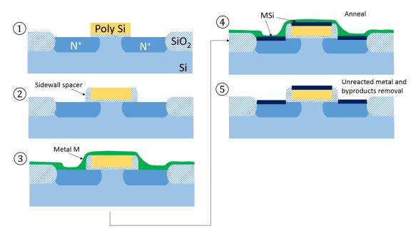
Figure 1.4 – Salicide process steps and formation of the intermetallics on Source/Drain (S/D) regions and on the gate of the MOSFET.
