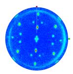
Figure 2.15 – Example of an in plane pole figure measured over a range of 90° over the  $\chi$  axis.
