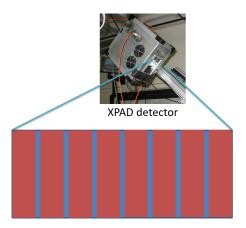
Figure 2.23 – Xpad detector and corresponding scheme of the modules arrangement in the detector.
