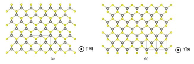
Figure 3.25 – A stack of InGaAs lattices projected along [110] in (a) and along the  $[\bar{1}10]$  direction in (b). As is represented by big gray spheres while In and Ga are represented by small yellow spheres. The unit lattice is marked by a rectangle on the figures.
