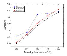
Figure 4.28 – Recalculation of the  $\alpha$  angle for ex situ annealed samples using the linear thermal expansion corrections.
