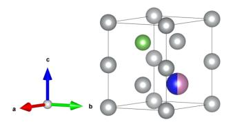
Figure 1.13 – Representation of a B8 Ni-InGaAs intermetallic with a stoichiometry of Ni $_4$ In $_{0.5}$ Ga $_{0.5}$ As. Grey atoms correspond to Ni atoms, green atom correspond to As, blue atom correspond to In and pink atom correspond to Ga. In this example, the B8 structure is fully filled and there are 2 atoms on the metallic sub-cell.
