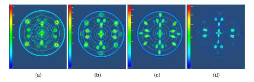
Figure 3.16 – Pole figure of the {1011} planes of the intermetallic hexagonal phase measured after the following annealings: (a) 300 °C, (b) 400 °C, (c) 450 °C, (d) 550 °C. The samples were measured using a Smartlab Rigaku diffractometer. Samples used are Ni(20 nm)/InGaAs/InP.
