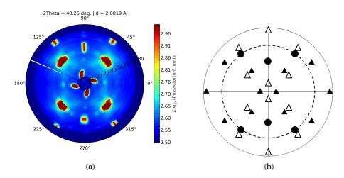
Figure 3.11 - (a) Pole figure of the  $\{10\overline{1}2\}$  planes of the intermetallic hexagonal phase measured after a 350 °C, (b) corresponding stereographic projection. The pole symbols are the same as defined in Table 3.1 and the dashed circle on stereographic projection represent the area that was actually measured. Samples used are Ni(20 nm)/InGaAs/InP.
