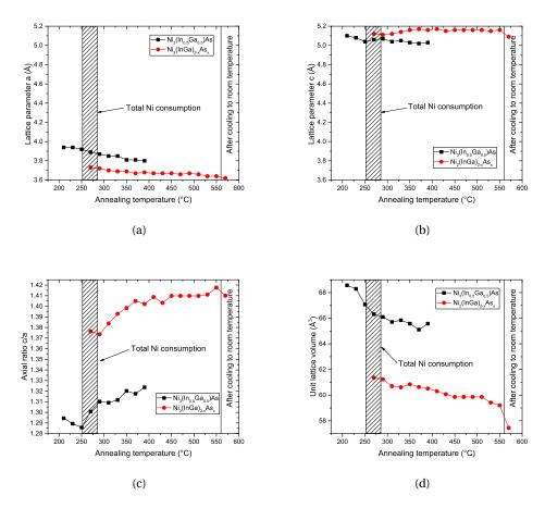
Figure 4.5 – Calculated parameters of the intermetallic hexagonal lattice (a) a lattice parameter, (b) c lattice parameter (c) c/a axial ratio and (d) volume of the hexagonal lattice. The used sample is Ni(20 nm)/InGaAs/InP.
