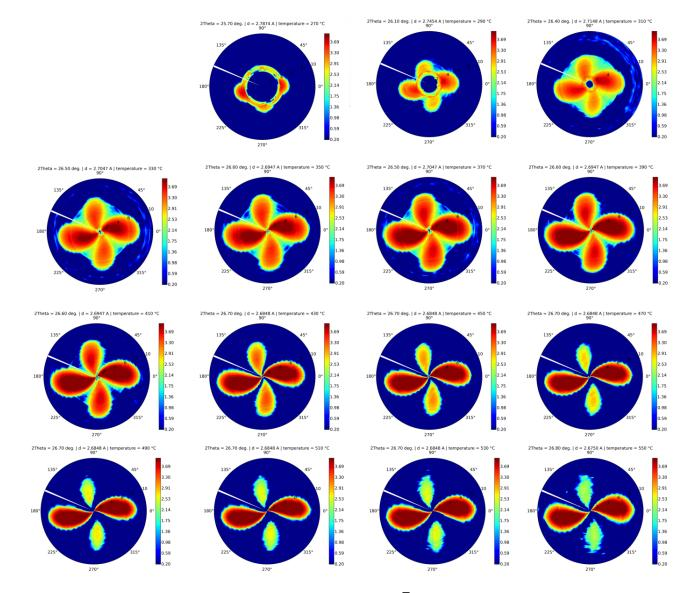
Figure 4.29 – Series of portion of the pole figures corresponding to the  $\{10\overline{1}1\}$  limited to  $\chi$  values between 0 and 10°. Each pole figure correspond to an annealing temperature starting from 270 °C and ending with 550 °C. The four poles in each pole figure correspond to the four  $\{10\overline{1}1\}$  planes that are located near the sample surface. The out-of plane region was not entirely accessible by measurement on the area detector for the first four pole figures.
