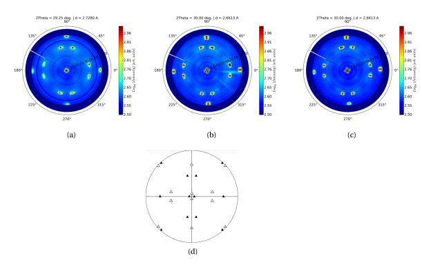
Figure 3.15 – Pole figures of the ntermetallic  $\{10\overline{1}1\}$  planes after an RTA annealing of (a) 350 °C, (b) 450 °C, (c) 550 °C and (d) stereographic representation of the pole figures. Samples used are Ni<sub>0.9</sub>Co<sub>0.1</sub>(20 nm)/InGaAs/InP.
