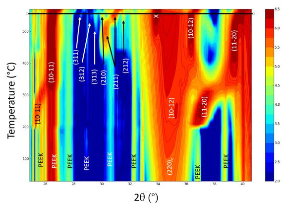
Figure 4.14 – Color map of the evolution of intensities according to  $2\theta$  angle and annealing temperature of the ramp for a Ni (7 nm)/InGaAs/InP sample. The bold black line at 550 °C denotes the measurement after slow cooling to room temperature. Sample used is Ni(7 nm)/InGaAs/InP.
