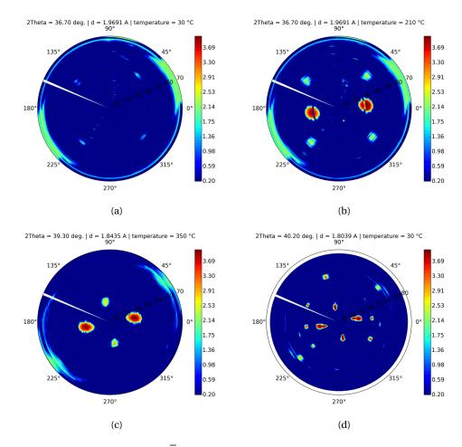
Figure 4.11 – Pole figures of the  $\{1\,1\,\overline{2}\,0\}$  planes of the hexagonal lattice, measured at 10 keV at different ramp temperatures (a) as-deposited (no intermetallic is formed yet), (b) at 250 °C, (c) at 350 °C and (d) at 30 °C after slow cooling to room temperature. The used sample is Ni (20 nm)/InGaAs/InP.
