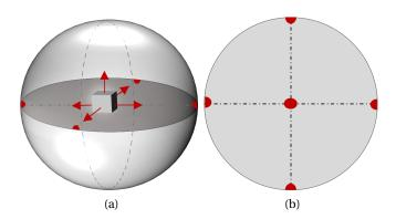
Figure 2.10 – Example of a stereographic projection of a cubic lattice with its  $\{100\}$  planes parallel to the surface:(a) Construction of the stereographic projection, (b) stereographic projection of the  $\{100\}$  planes.
