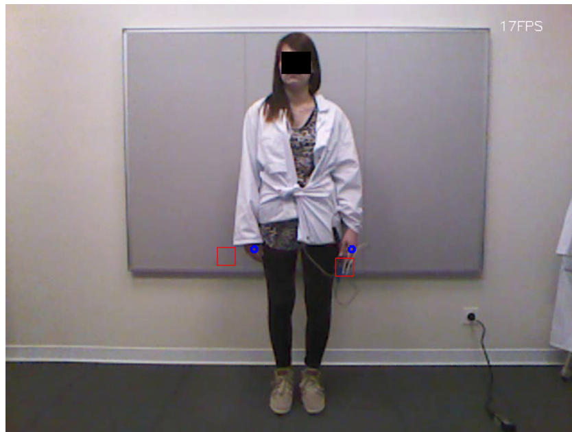
Figure 4.4: Example of the refinement of the hand joint location. The red squares represent the location given by the Kinect. The blue circles represent the new location after refinement. Best viewed in color.
