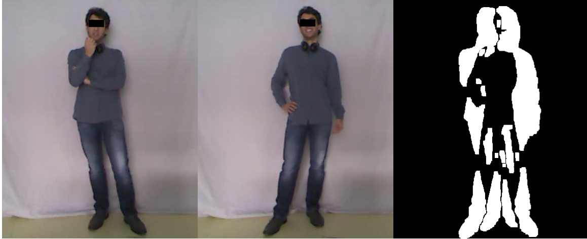
Figure 4.3: Example of detection of a posture change. From left to right: first frame of the period, last frame and their thresholded absolute difference.
