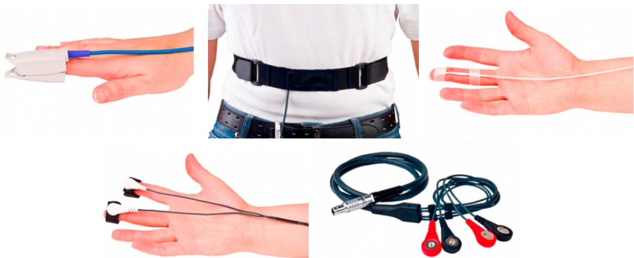
Figure 4.7: Images of the sensors used to capture physiological signals. Top row, from left to right: BVP sensor, respiration sensor and temperature sensor. Bottom row, from left to right: skin conductance sensor and EXG sensor 2 .
