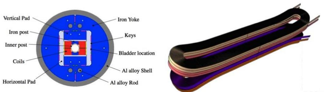
Figure 1.15 Design of FRESCA2 LTS outsert using  $Nb_3Sn$  in 2D at straight part (left) and in 3D magnet ends (right) [37].
