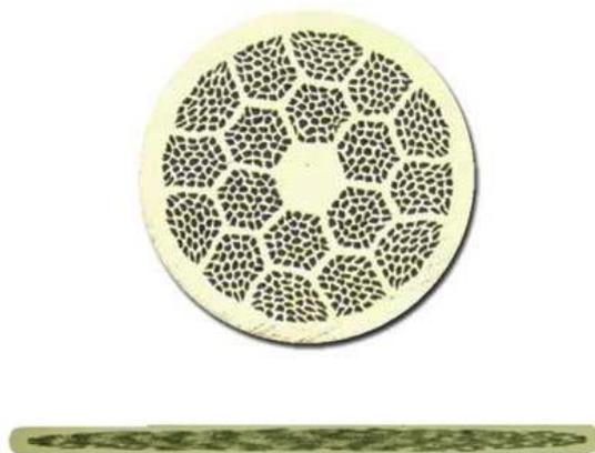
Figure 1.16 Cross-section of Bi-2212 wire with power-in-tube process [43] and Bi-2223 tape [44].
