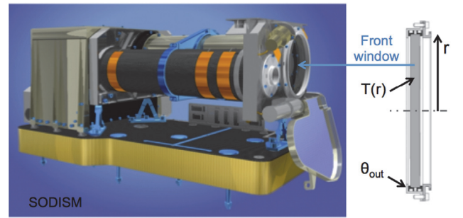
Figure 3. Location of the front window at the telescope. \theta_{out} represents the front window interface temperature, and r is the radial coordinate.
