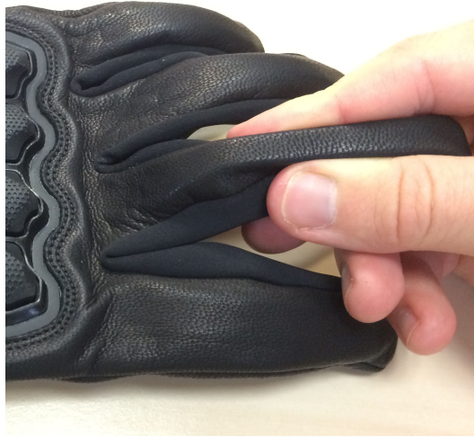
Figure 5.8: The flex sensors are fully integrated between the glove's inner and outer layers.
