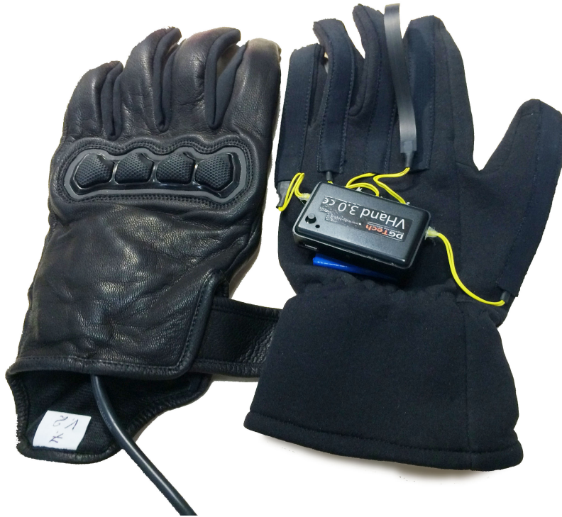
Figure 5.2: Our custom glove and the V-Hand, for comparison. One V-Hand flex sensor was put out for visibility. Despite integrating similar sensors, our glove arguably suits outdoors conditions better.
