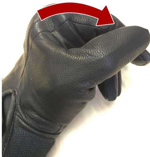
Figure 5.4: Sliding is sensed thanks to a Hall effect sensor and two alternating magnets. Given the consecutive signs of magnets, the glove reports the sliding direction.
