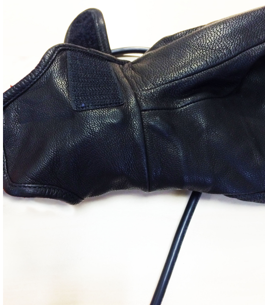
Figure 5.5: The vibrating motor (small circular piece below the strap) is put against the wrist for best sensitivity by the operator.
