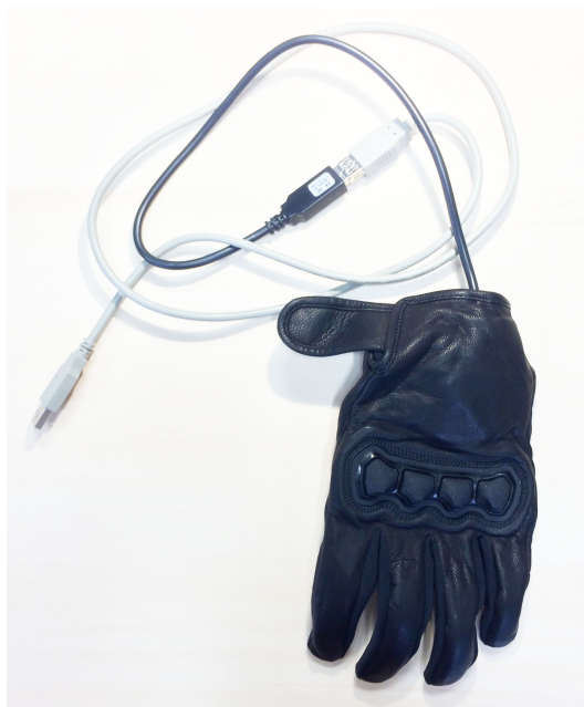
Figure 5.3: The glove with a simple USB extension cord. This gives enough length for connexion into a device in the operator's pocket or near their belt, making the extension cord pass in their sleeve. One could also imagine a smart vest in which a receiving USB port is directly made available at the end of the sleeve, bypassing the extension cord altogether.
