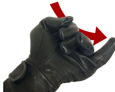
Figure 4.16: Gesture "lock" would then disable the robot control to protect against recognition mistakes.
