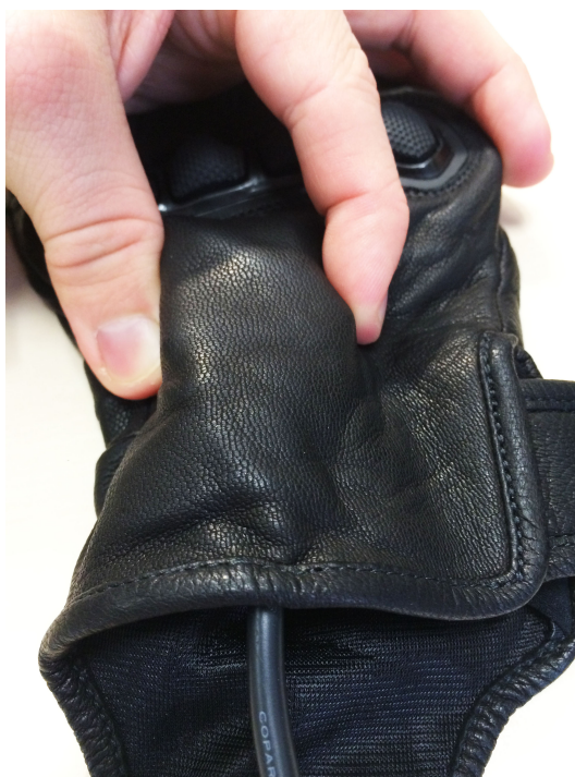
Figure 5.7: The ArduIMU board is very light and is not felt by the user. It is protected between two glove layers.
