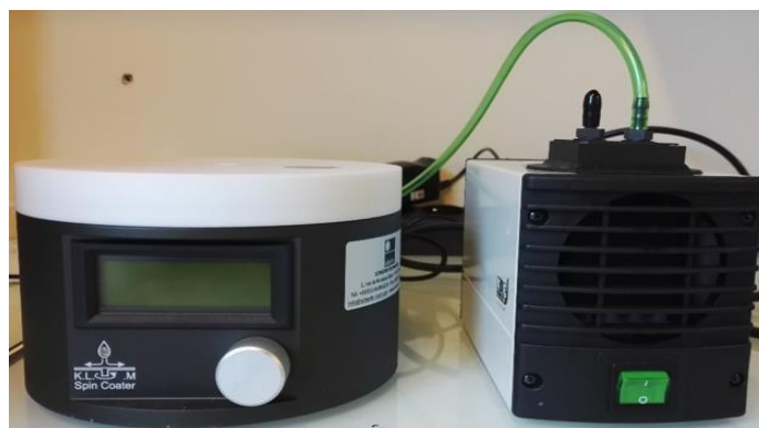
Figure 2.12 SCC-200 spin coater (left) and coupled pump for vacuum (right) (Laboratoire de Chimie Physique, LCP, Paris-Sud University).
