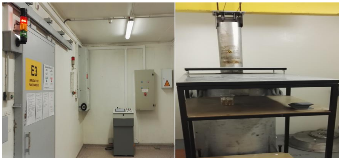
Figure 2.7 Photograph of ^{60}\text{Co} gamma source (LCP, Paris-Sud University). Control panel (left) and irradiation plate (right).
