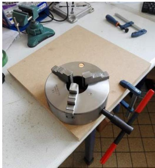
**Figure 5.4:** Circular three-jaw self-centering chuck mounted on a wood plank, used for holding the bone stable.
