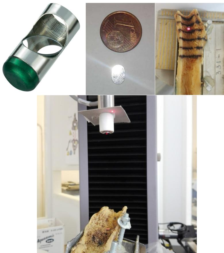
**Figure 6.7:** From left to right (top): mirror of an endoscopic camera - VOLTCRAFT - 4,5 mm diameter (top left and middle - Source: <http://www.fonetip.cz/>). Laser beam pointed at the mirror placed on the bone's surface on a test spot. Laser beam reflected back to the beam's source with the mirror to verify orthogonality (bottom).
