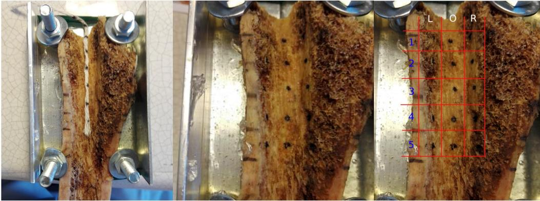
**Figure 6.8:** Different steps for the definition of indentation spots. A fine rope with evenly separated marks is used to make the grid (left). A permanent marker is used to mark the spots for the indentation, 3 columns, and 5 rows (middle). Reference names are associated to each spot with numbers from 1 - 5 for the rows, and the letter L, O and R for the columns (right).
