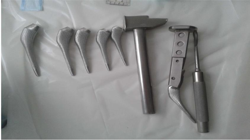
**Figure 1.5:** Broaching tools (Symbios®) of different sizes used for THR.
