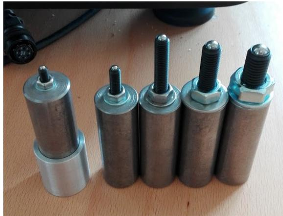
**Figure 6.4:** Set of screwed indenters ranging from M4 to M24 (indenter diameter 2,5 mm to 18 mm).
