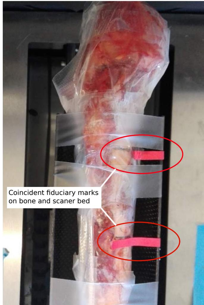
**Figure 5.6:** Coincident reference lines, on bone (black lines), on scanner bed (red tape), for sample positioning in the scanner.
