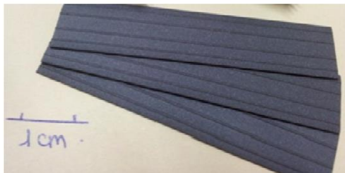
Figure II-6. Extruded profiled plates made of 91.5 wt% of magnetocaloric powder and 8.5 wt% of polymer.
