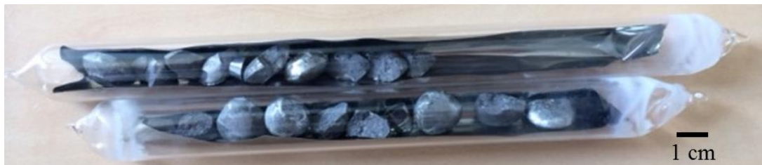
Figure II-3. Example of sample preparation for high temperature annealing.
