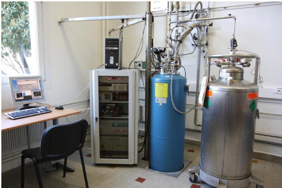
Figure II-9. Schematic representation (top) and photo (bottom) of the extraction vector magnetometer for low-temperature range at the Néel Institute.
