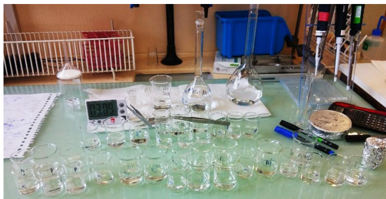
Figure 83 - Line of becher for layer by layer deposition and rinsing between each layer.
