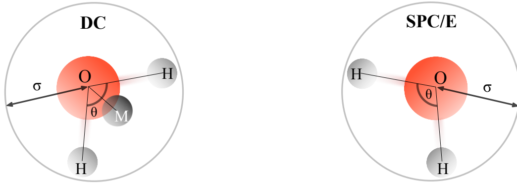
Figure 3.1: Geometries of the Dang and Chang (1997) models (DC, left) and of the SPC/E (Berendsen et al., 1987) water model (right). The size of the repulsive Lennard-Jones core is given by \sigma . The angle \theta \approx 105^\circ is close in value to the ideal tetrahedral angle. The OH distance is close to 1 Å. The M site is fictitious and may host the molecular dipole.
