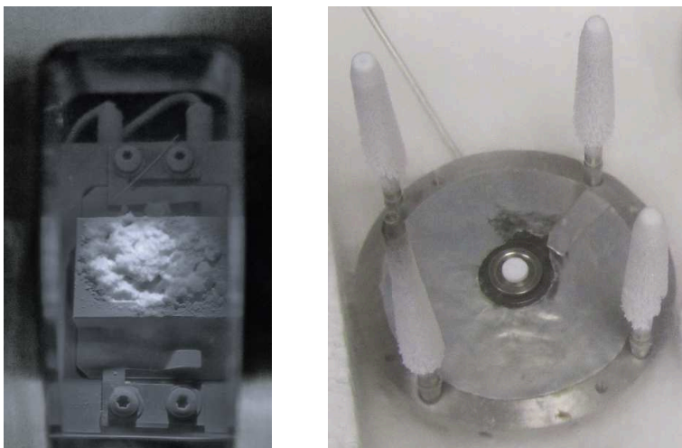
Figure 4.6: Left: powder sample of quenched \text{NaCl} \cdot 10.2\text{D}_2\text{O} solution inside the cryochamber in the XRD at IMPMC. Right: pellet ( \varnothing \approx 1.8 \text{ mm} ) of amorphous powder loaded in a gasket on an anvil of the Paris-Edinburgh cell. (Ludl et al., in preparation)
