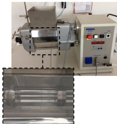
Fig. 2.5. Erweka AR 402 milling device
