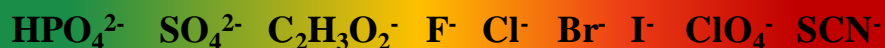
Figure 1.16: Hofmeister series: ranking of anions by their hydration degree. The hydration degree is decreasing from the left to the right of the scheme.
