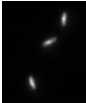
Figure III-7: At high concentration of PI, Neo-Cy5 and PI fluorescent signals can be discriminated.
