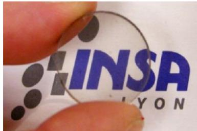
**Figure 1.20.** Micrograph of a sintered MgAl<sub>2</sub>O<sub>4</sub> spinel [Bonnefont 2012]
