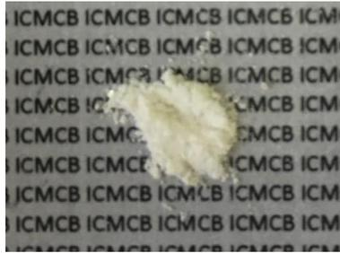
**Figure 2.27:** SPS pellet issued from a powder heat-treated under a flame.
