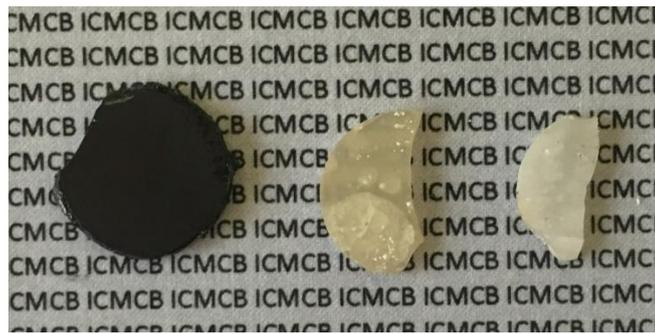
**Figure 2.26:** SPS pellets: as-sintered (left), heat-treated under oxygen at 900°C during 6h under  $O_2$  (medium) and additional treatment at 1300°C 2h in air (right).
