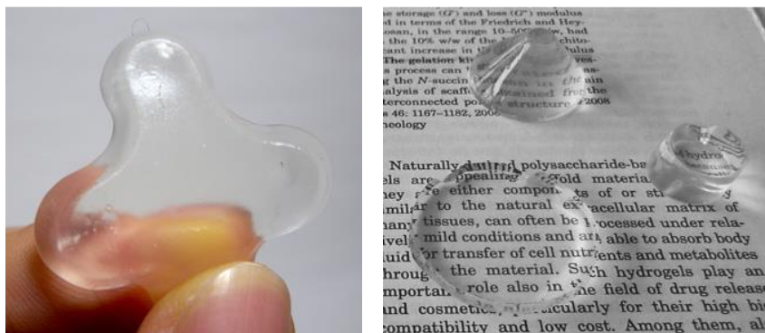
Figure 1.1 Example of transparent high-water-content hydrogel of different molded shapes. Left: adapted from Q. Wang et al., Nature , 2010 , 463, 339-343; right: adapted from M. C. Straccia et al., Carbohydrate Polymers , 2015 , 125, 103-112.
