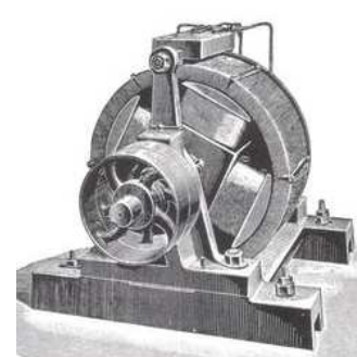
Figure 1.3 : Machine synchrone de Haselwander, 1887 [Kit17]
