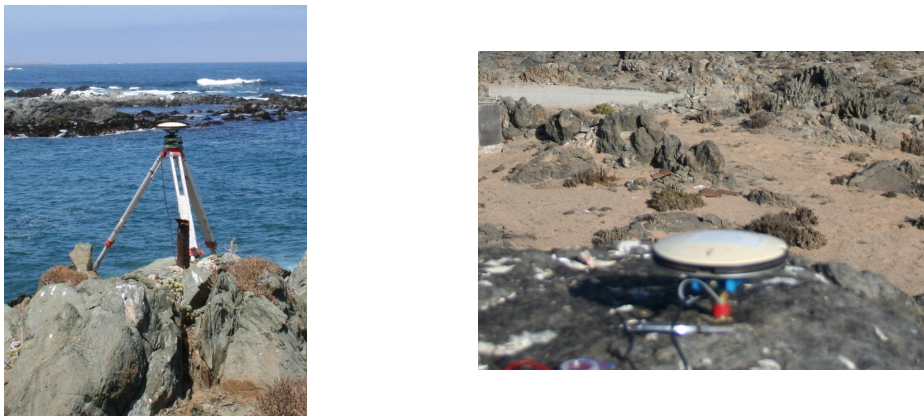
FIGURE 2.10 – Gauche : Measurement with tripod - marker PTOM; Droite : drilled monument in bedrock - marker CZBA
