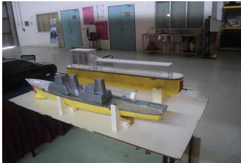
Figure 4.21 Both models fixed with rod before the test
