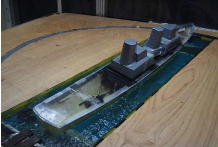
Figure 4.28 The rotating table is turned 15^\circ to simulate the wind direction from port 105^\circ
