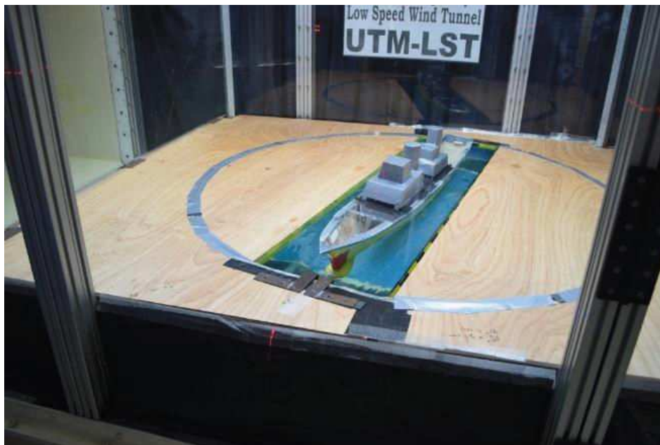
Figure 4.27 The rotating table is turned 15° to simulate the wind direction from starboard 75°
