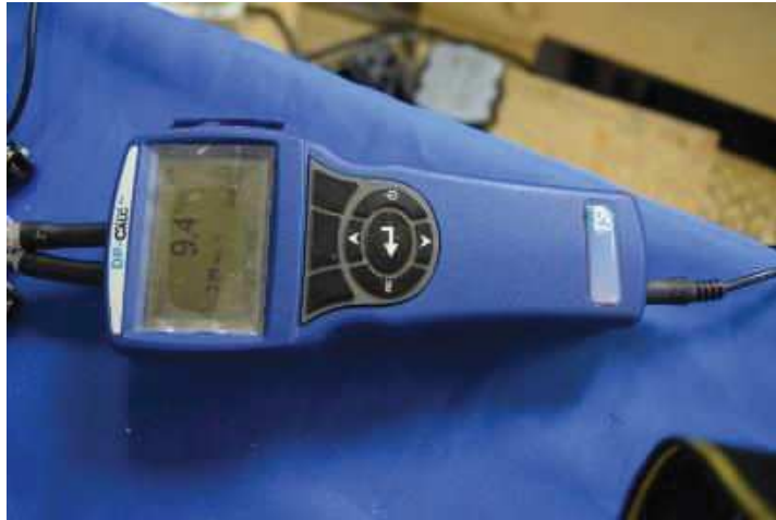
Figure 4.18 DP-CALC Micro manometer 5825 used to verify the wind velocity in the test section
