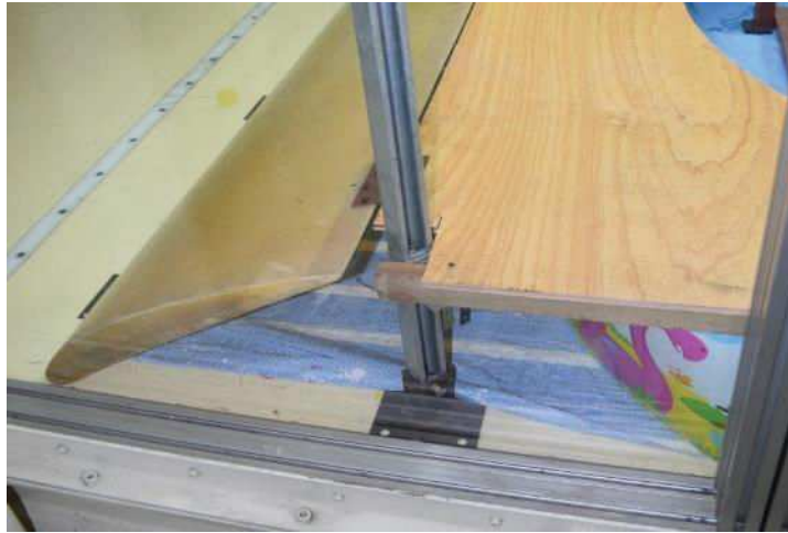
Figure 4.15 Side view of test section with spoiler and dummy test section floor
