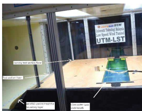
Fig. 8 Arrangement in the test section
