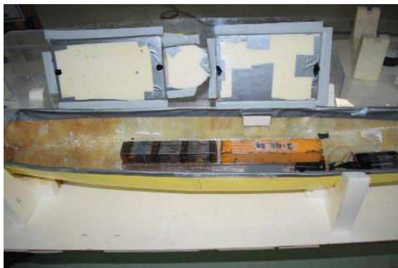
Figure 4.20 Arrangement of loads and accelerometer in the model hull
