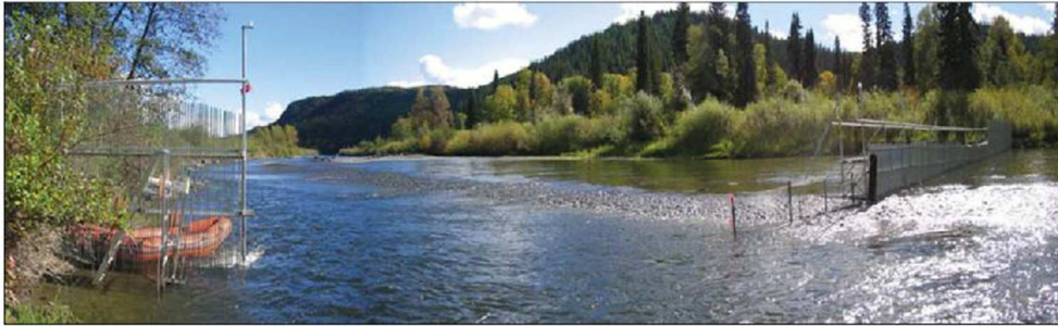
Figure 14 Cross-section of a DIDSON hydroacoustic site on the Horsefly River (Canada), using a deflector weir. Photograph by J. Lilja (Cronkite et al. 2006).
