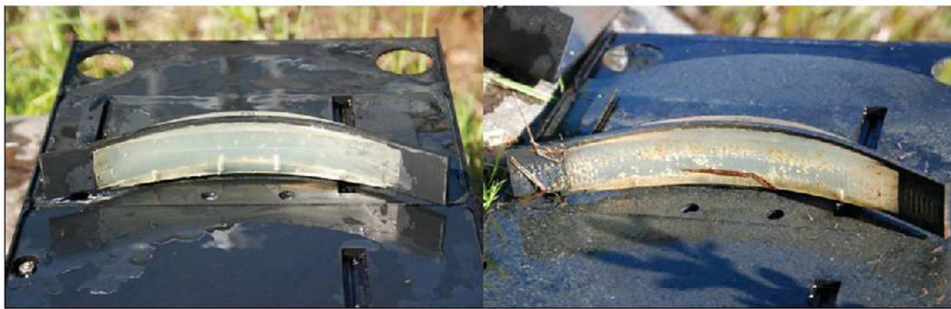
Figure 11 Photo of the DIDSON lens: clean (left) and covered by drifting pollen (right) (Lilja et al. 2010).
