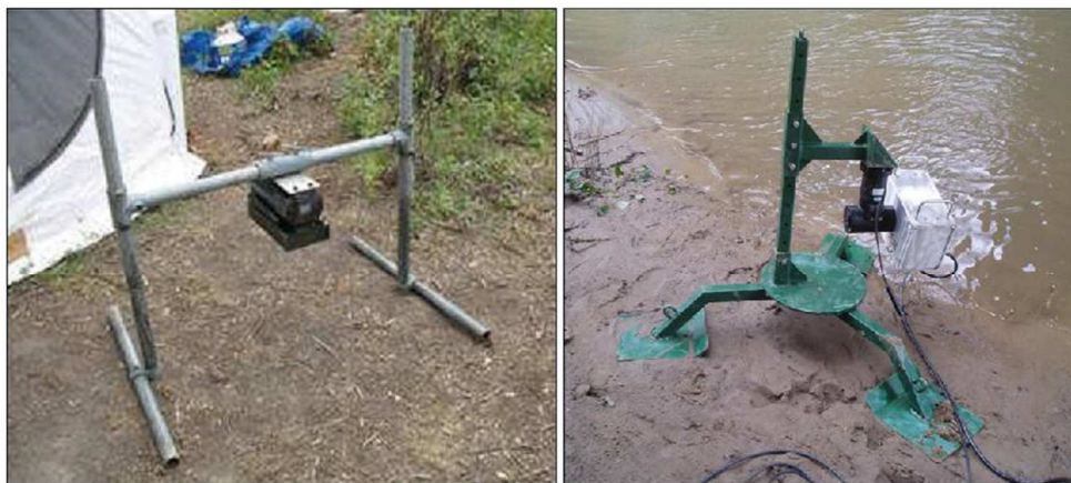
Figure 13 Two different DIDSON fixation supports: left: an aluminium H-mount (Mercer and Wilson 2009); right : a tripod-style DIDSON mount (Pipal et al. 2010b).
