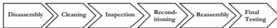
Figure 6. An example of a generic remanufacturing process, based on the five key steps described in Steinhilper (1998).
