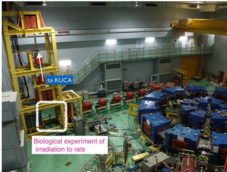
Figure 1.8: FFAG complex at KURRI [21]: the extraction line is shown in the background. The 150 MeV FFAG is the larger of the two rings.
